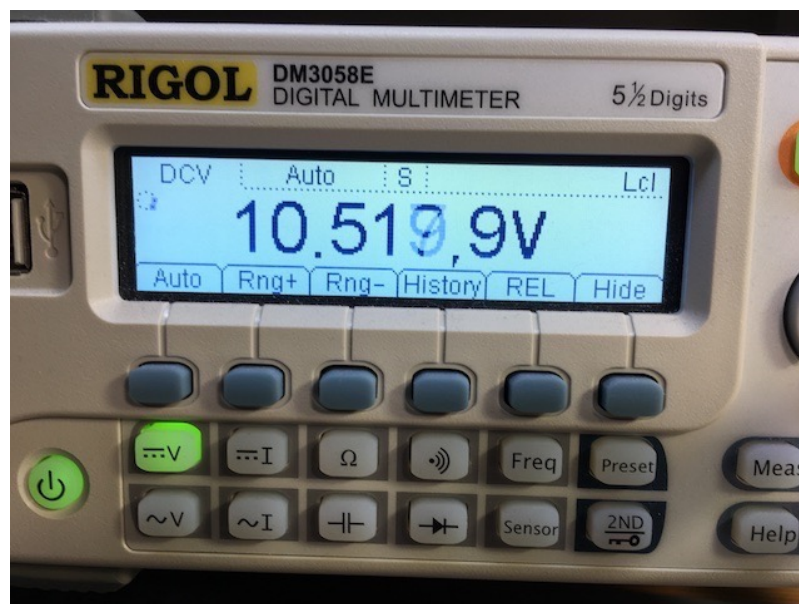
Figure 17.5: The actual voltage of the 9 V DC mains power supply I use to power the breadboard power supply.
