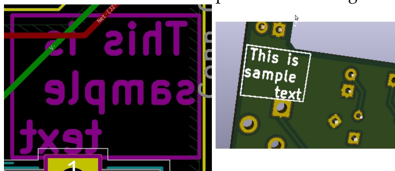
Figure 28.12: The text and box appear in the bottom silkscreen.
