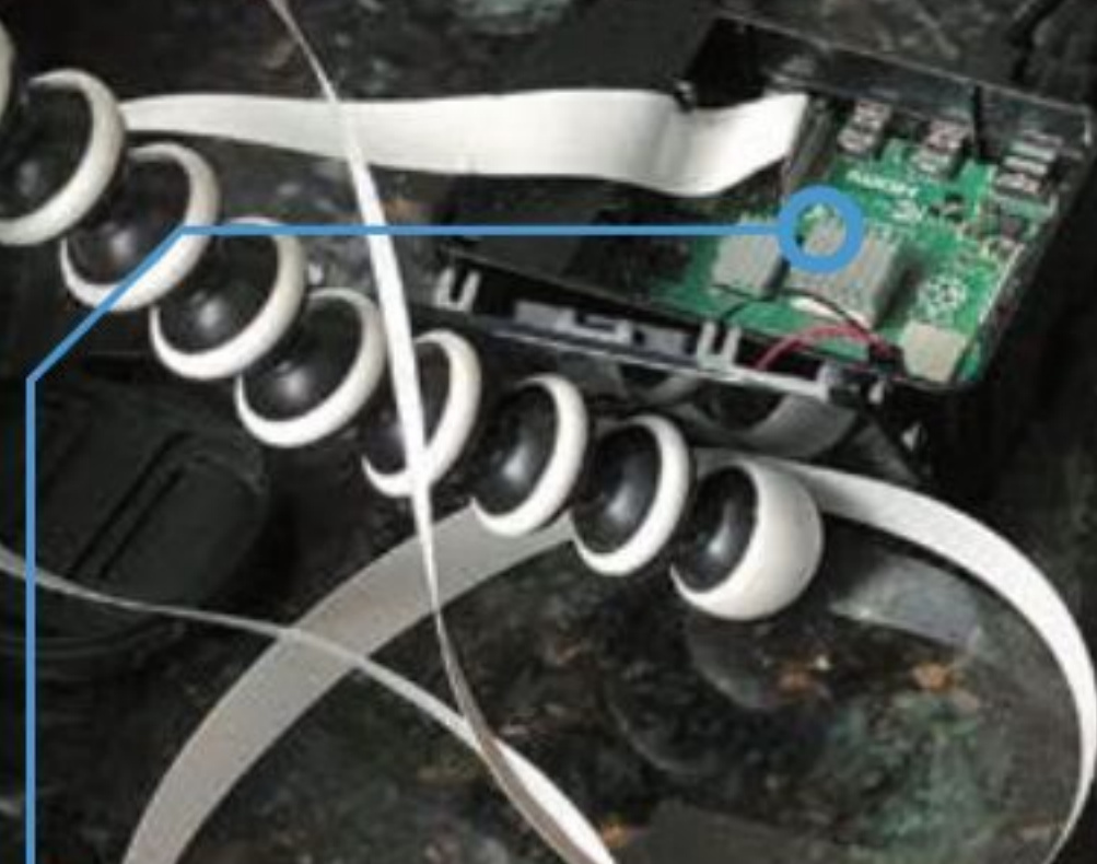
Running on a Raspberry Pi 4, PI-TIMOLO detects motion and then captures an image
