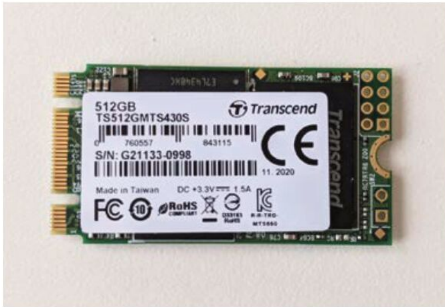
▲ A Transcend M.2 SSD drive with a SATA III connection (on the left)
