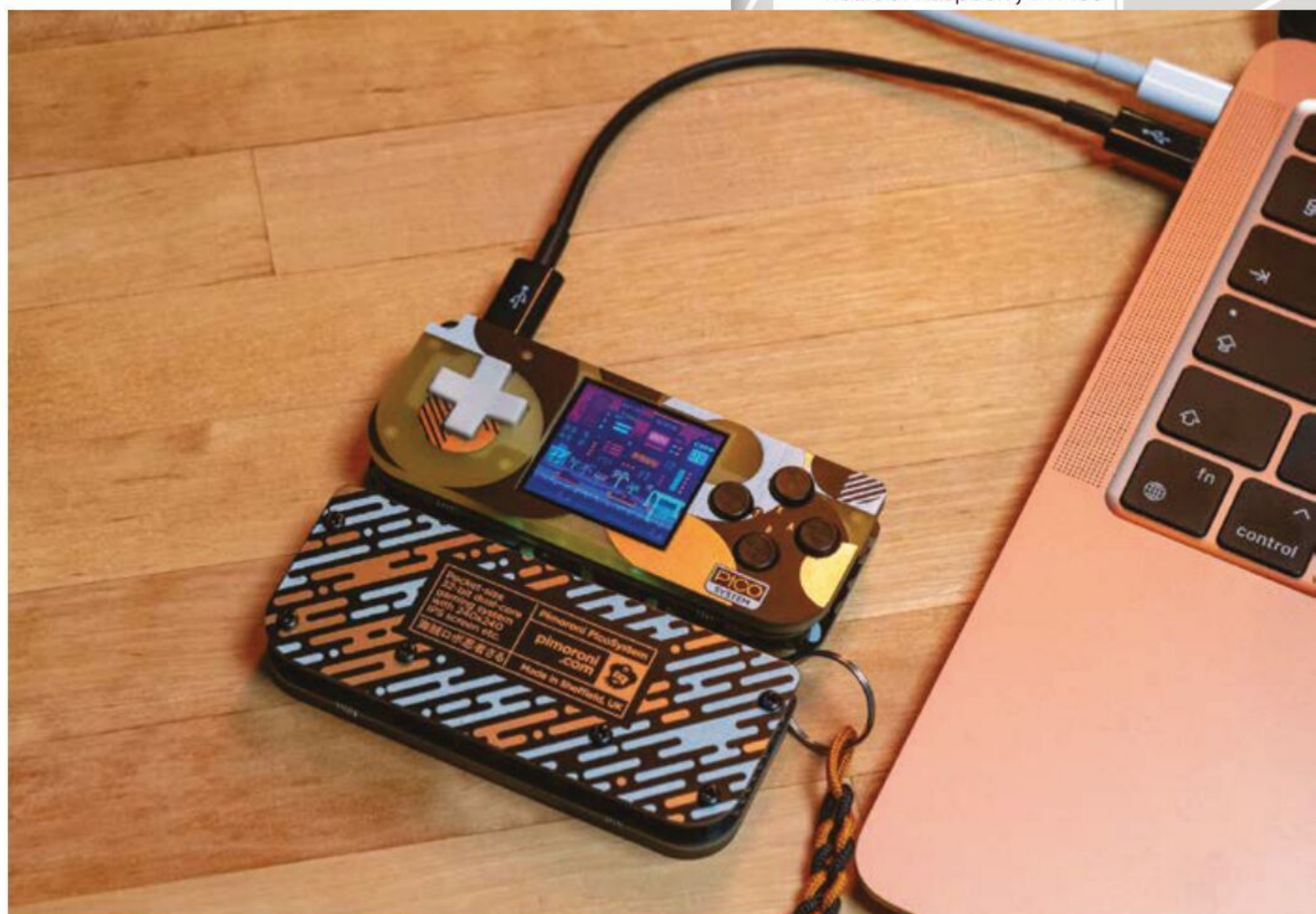
▼ PicoSystem is an all-in-one games console based around the powerful RP2040 microcontroller at the heart of Raspberry Pi Pico
