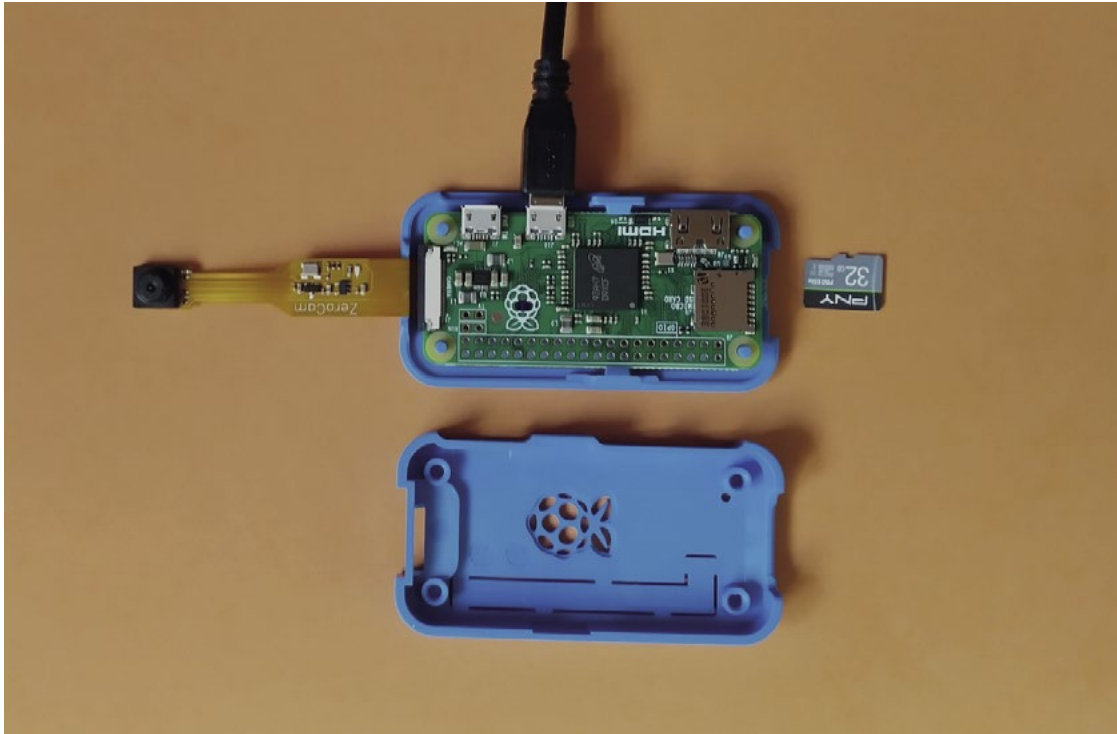
◀ A Raspberry Pi Zero with ZeroCam is fixed to the ceiling above
