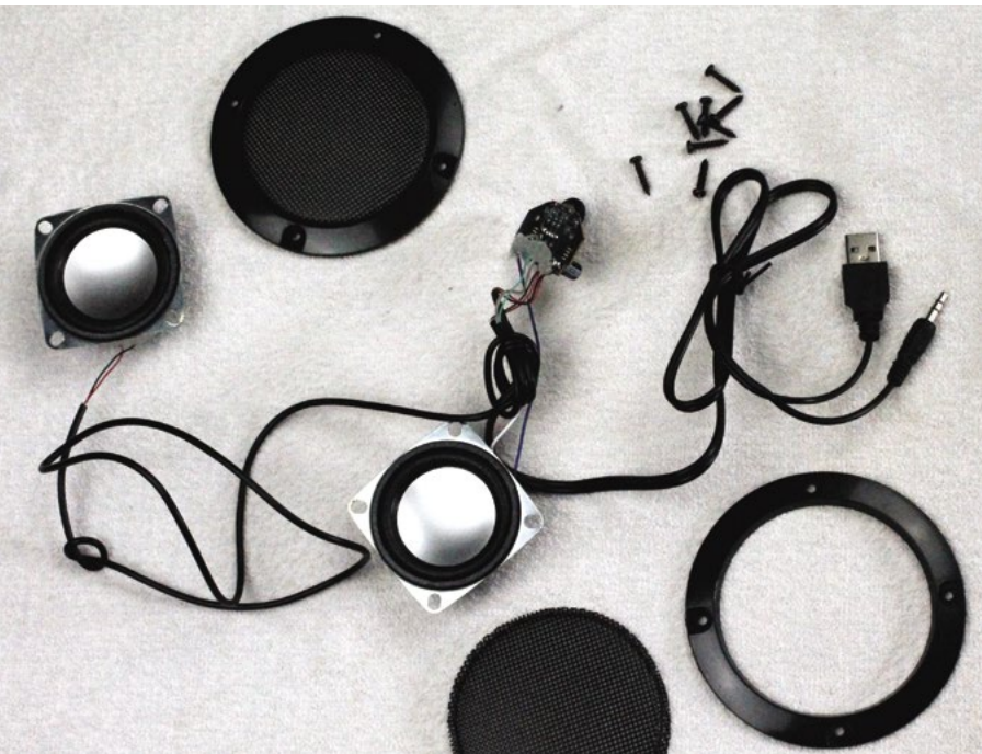
▲ A variety of compact bus- and mains-powered amp and speaker kits are available: this one takes power from the USB port and audio from the 3.5mm port
