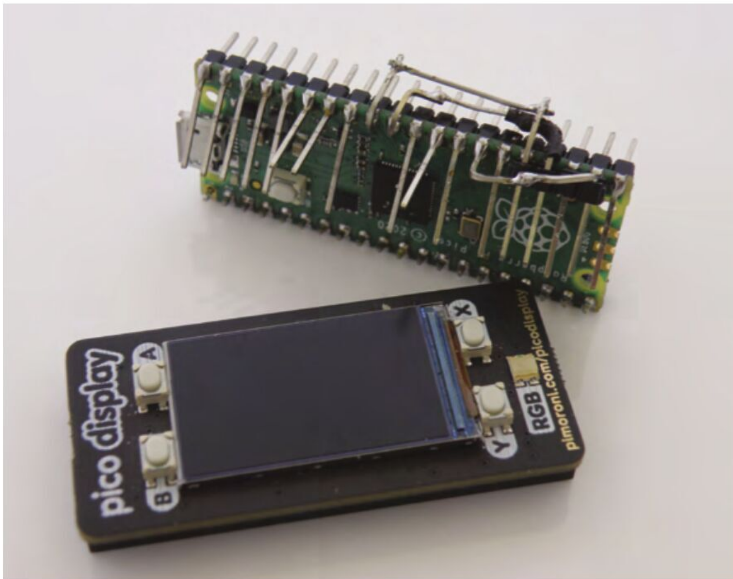
▲ A certain amount of adjustment to the header pins was needed
