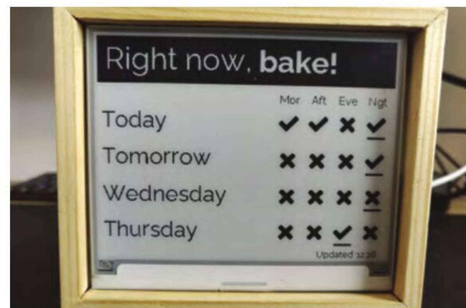
▲ Using his ShouldIBake project, Andrew schedules sourdough loaf baking when the maximum amount of energy to heat the oven comes from renewables
