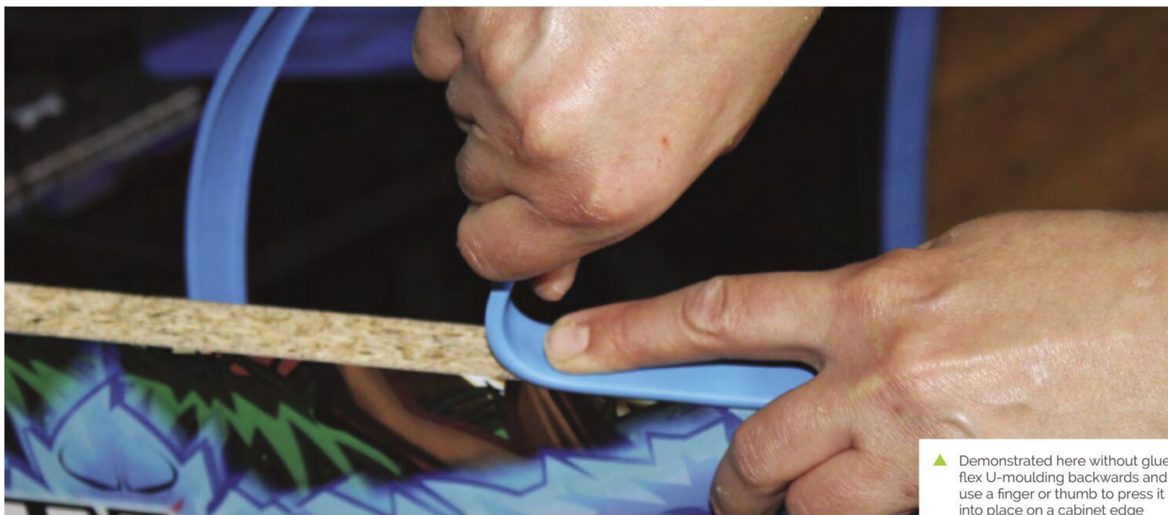
▲ Highly flexible, U- and T-moulding are used to give a clean finish to the cabinet edges
