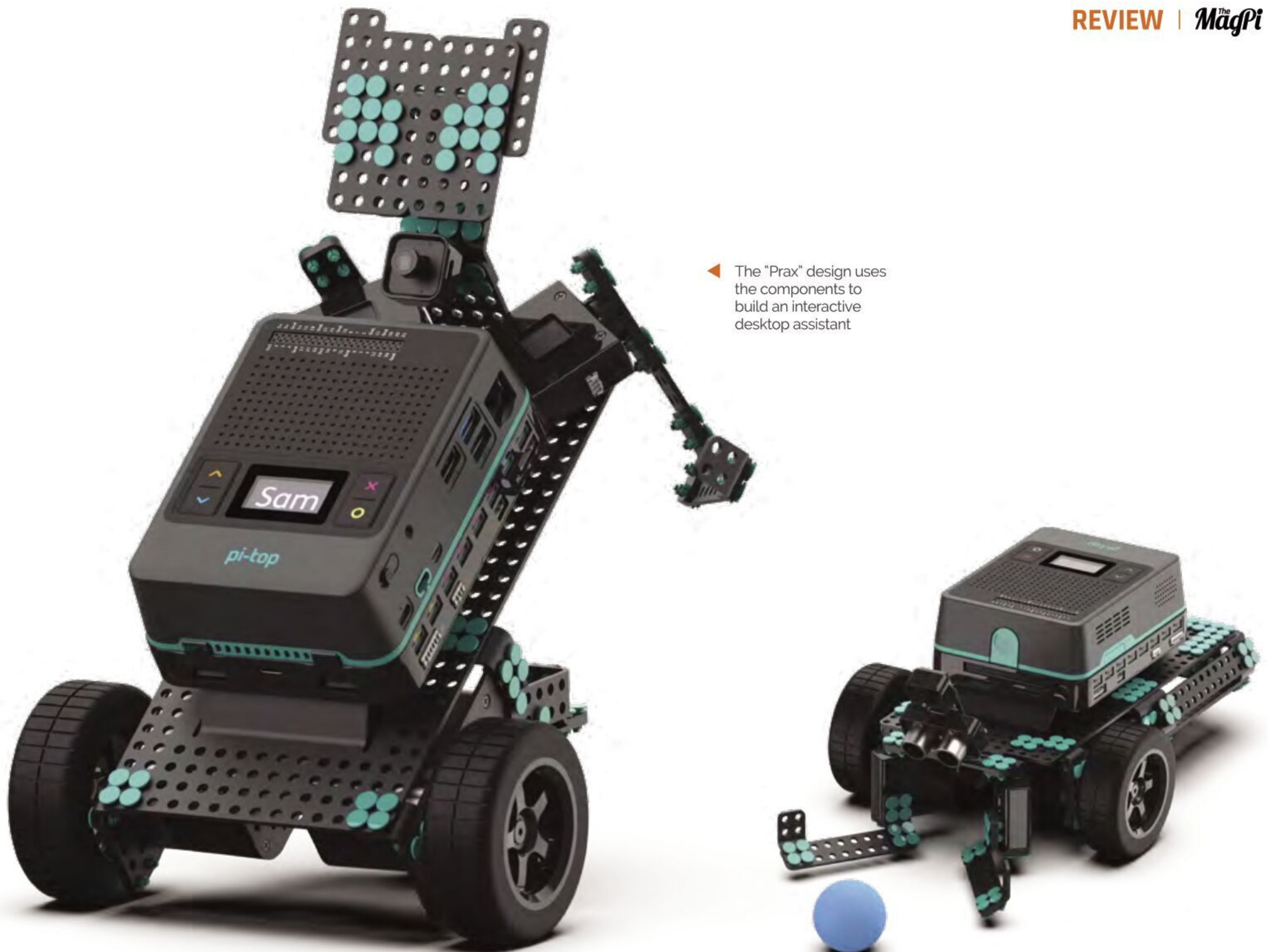
▲ The pi-top Robotics Kit designs are sturdy. The "Bobbie" design uses servo motors as two pincer arms
