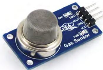
▲ The MQ-5 gas sensor can detect several noxious gases in the air and is highly sensitive
