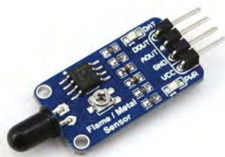
▲ The Waveshare flame sensor has both analogue and digital outputs. Sensitivity can be adjusted with the screw
