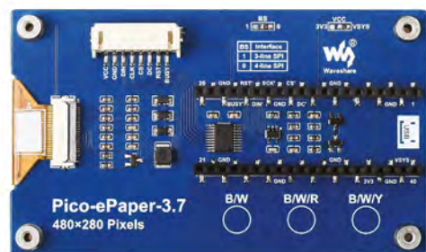
▼ The rear features female headers to insert a Pico, plus an SPI interface to connect other boards
