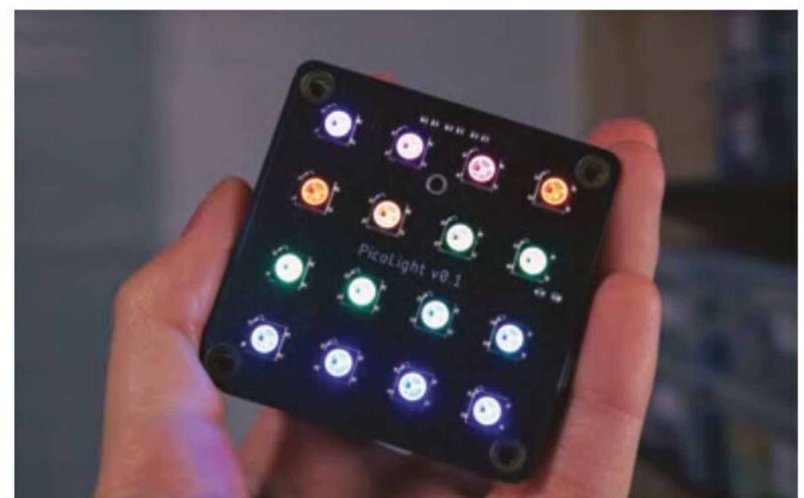
▲ The 4×4 NeoPixel matrix in rainbow cycle mode
