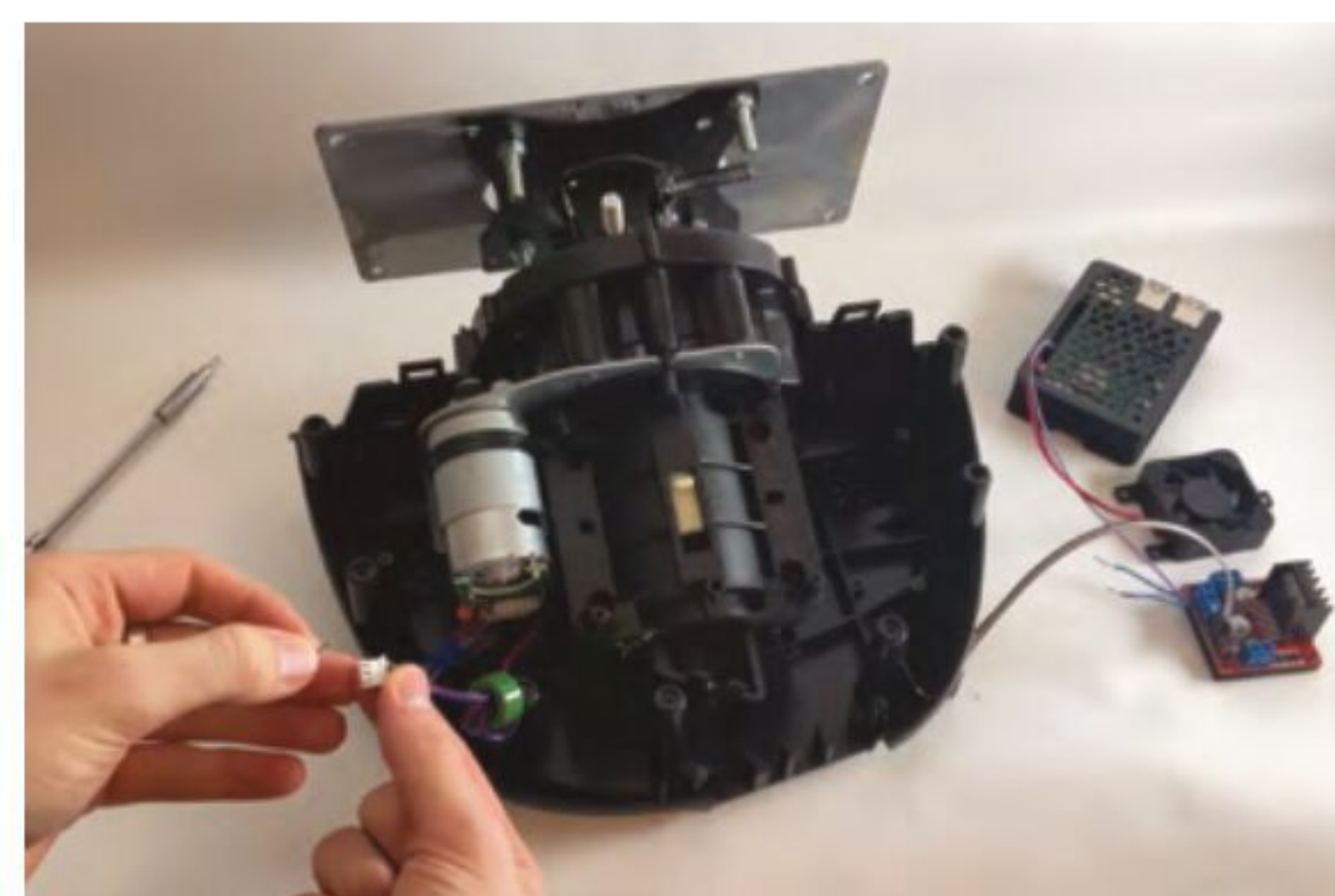
▲ A major challenge was to fasten the VESA mount so that it can withstand the emerging torque when swinging a TV
