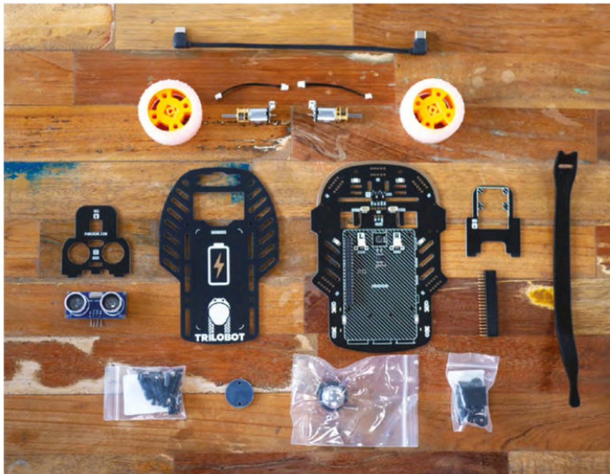
▲ The components supplied in the Trilobot Base Kit. Just add a Raspberry Pi, microSD card, power bank, and Camera Module (optional)
