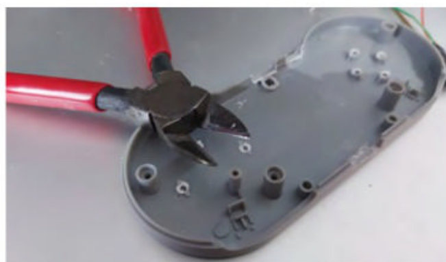
^ Figure 11: We can now start to trim away the unwanted pieces of plastic from the two halves of the case.
