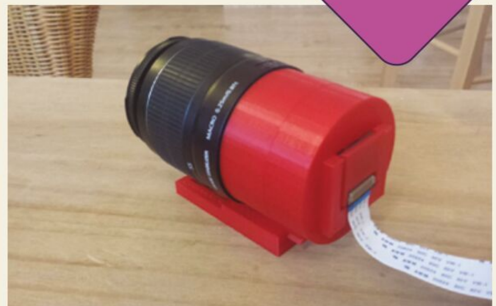
▲ Using a 3D-printed lens adapter, you can use powerful lenses with a standard Raspberry Pi Camera Module
