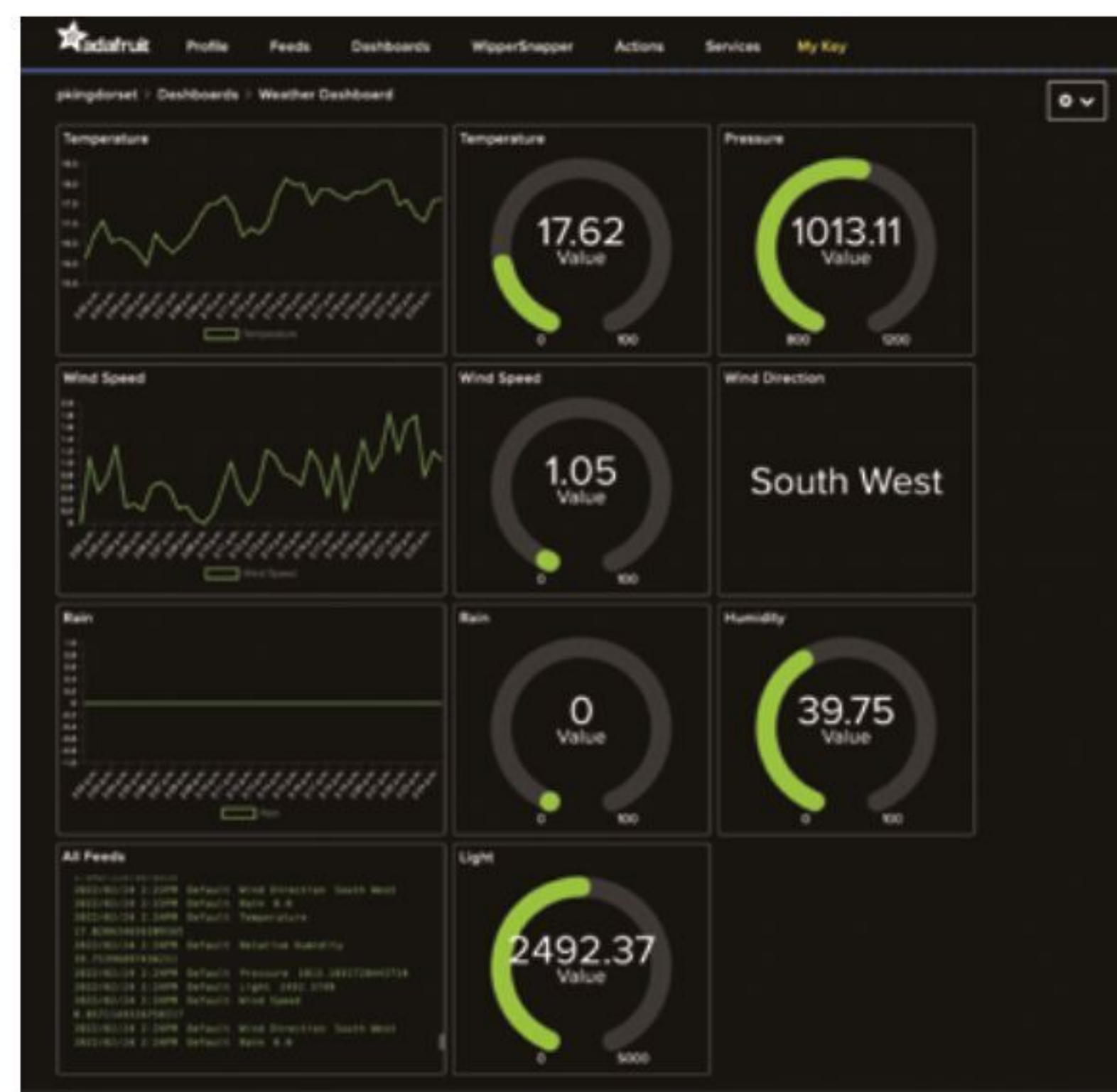
▲ It's very easy to hook your weather station up to an Adafruit IO web dashboard to log all the data there
