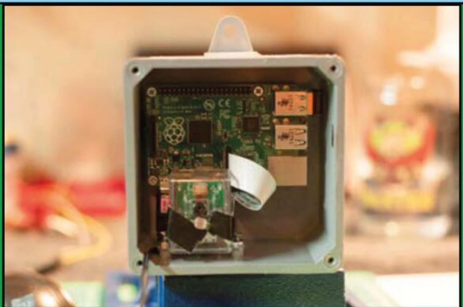
▲ Building your system to be waterproof is very important
