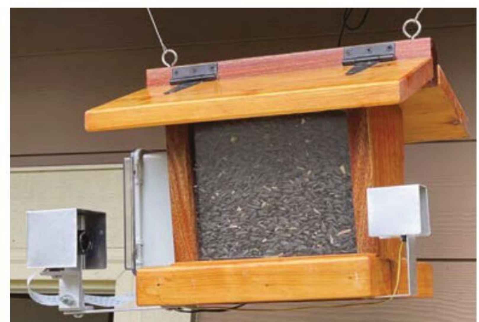
▲ The camera and ultrasonic sensor are set on either side of the area where birds will feed
