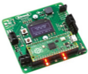
▲ The BME688 sensor is at the top left of the board; its readings can be shown on a small OLED in the middle
