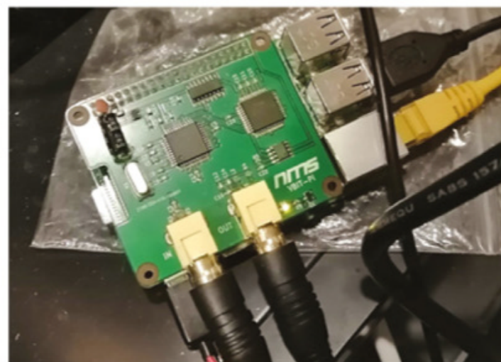
▲ Nathan has designed his own VBIT-Pi 3 board which adds a teletext stream to a PAL video signal
