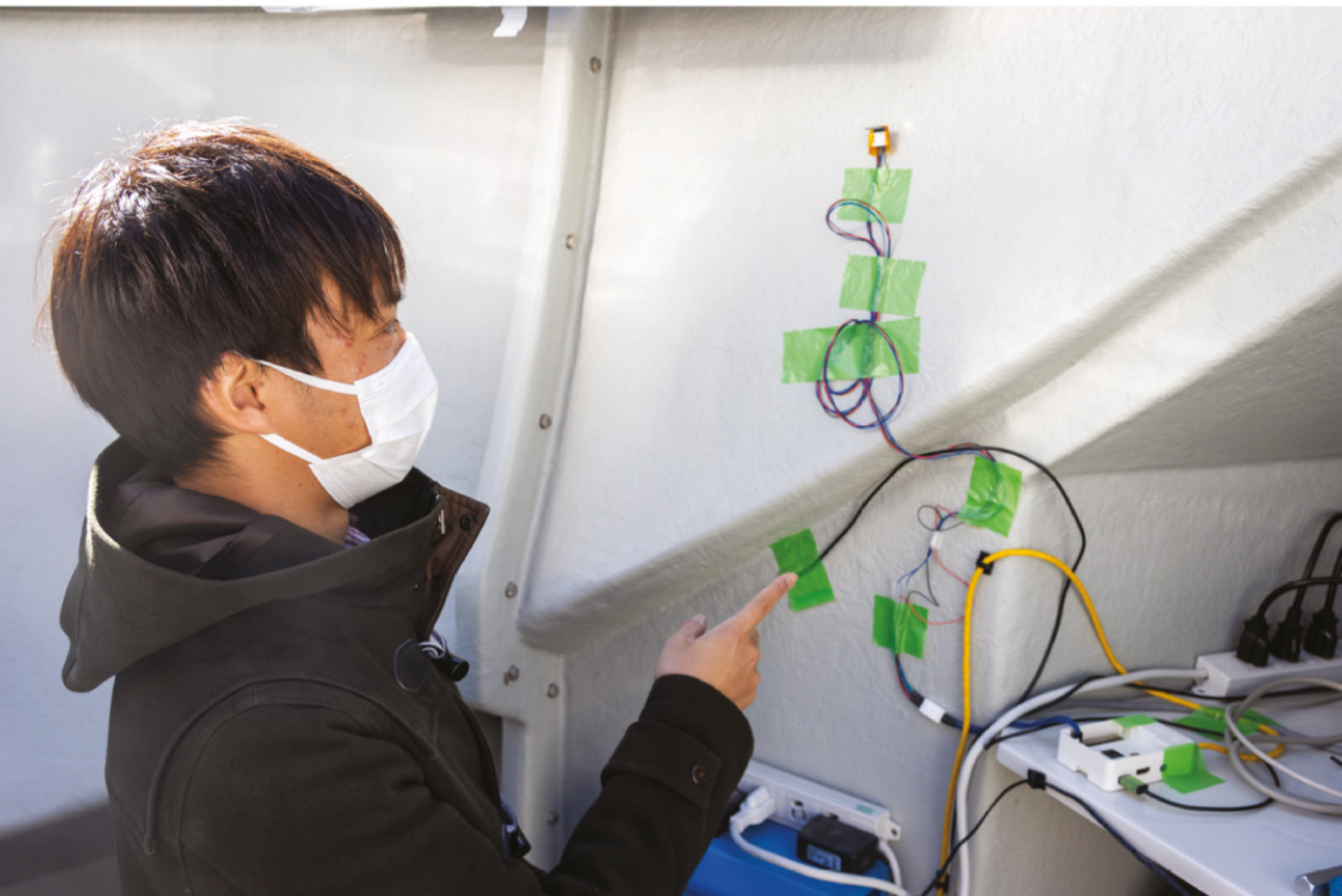
▲ Shunsuke Honda points out the pera-pi Raspberry Pi sensor checking on the humidity and temperature within the telescope dome
