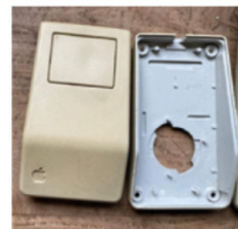
▲ The keyboard and mouse were originally yellowed, but Dan took them apart and used a home-made chemical mixture to whiten them
