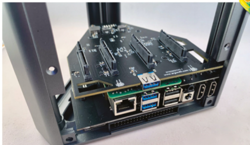
▲ Argon EON cases can hold several hard drives at once for an excellent NAS
