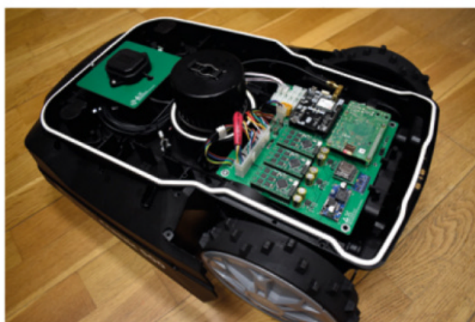
▲ A Yard Force Classic 500 mower was used as a base for the project, providing the required motors and mowing components in a neat package
