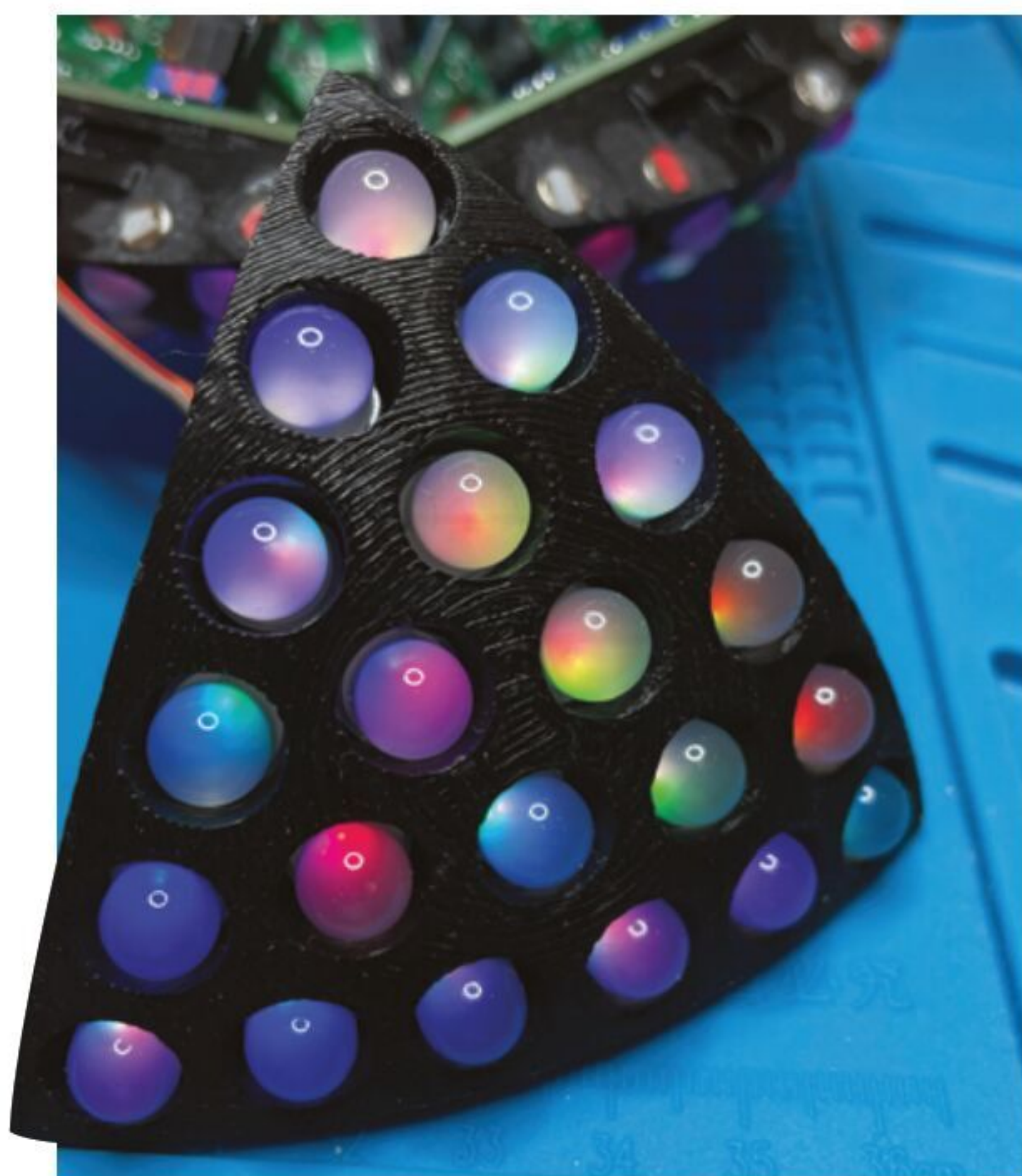
▶ A sphere element containing 21 LEDs. "You need to insert the LED through the sphere element, then try to fit each of its four metal leads through a very tiny 0.85 mm diameter hole," Tom explains
