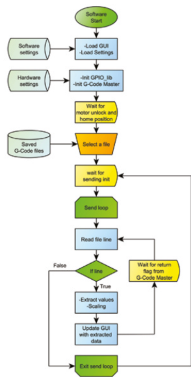
▲ Figure 1: A flowchart showing the software process: G-code is translated into coordinates to set the movements for the motors
