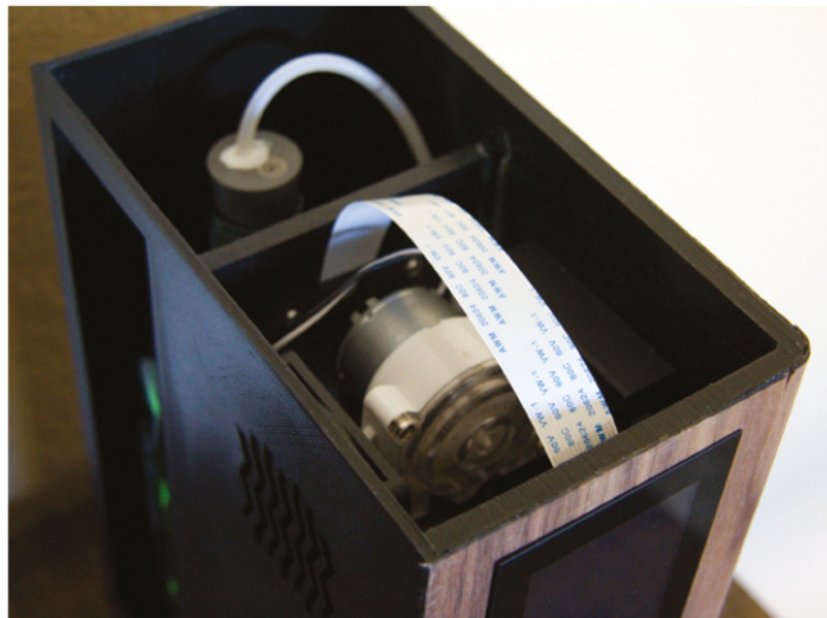
◀ Raspberry Pi powers the various pumps and sensors, and also connects to a custom PCB for the project
