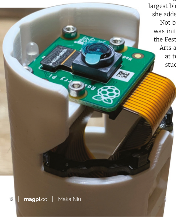
◀ A Raspberry Pi Camera Module V2 fits neatly at the end of the project’s housing
