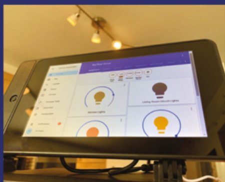
▲ View and control your smart home appliances on the Home Assistant web dashboard
