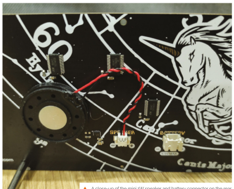
▲ A close-up of the mini 1W speaker and battery connector on the rear
