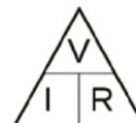
▲ Figure 3 The Ohm's law triangle, makes it easy to find the formula for calculating resistance, voltage, or current
