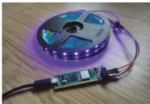
▲ The Plasma Stick uses the power of the RP2040 chip's PIO capability to drive LEDs at a high, flicker-free frame rate
