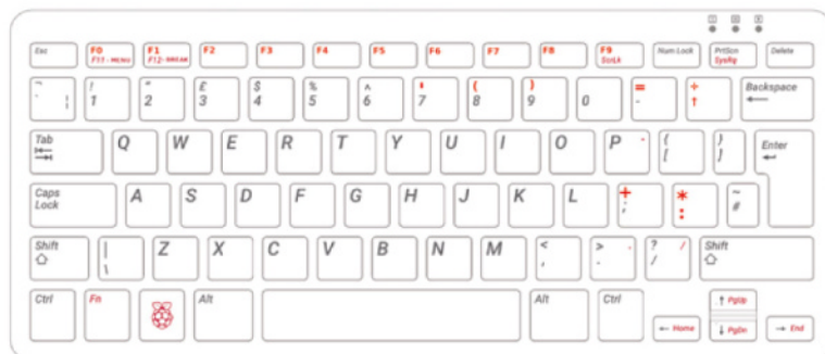
Figure 1 BBC Micro keyboard map for the UK Raspberry Pi keyboard. BBC keys are marked in red
