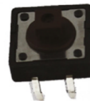
▲ Figure 6 Many switches have four pins. The pins on each side are connected together, with the switch going between them
