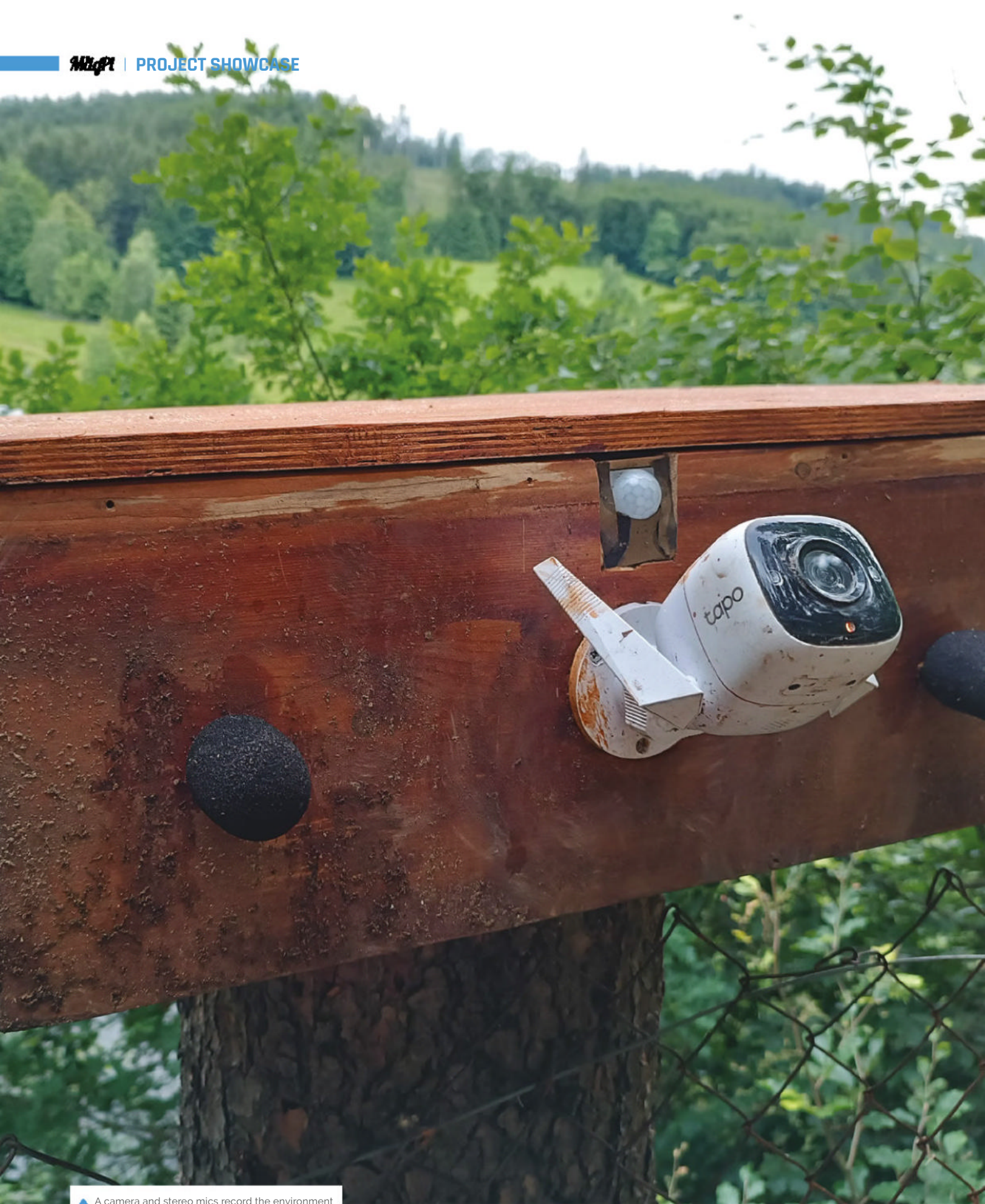
▲ A camera and stereo mics record the environment
