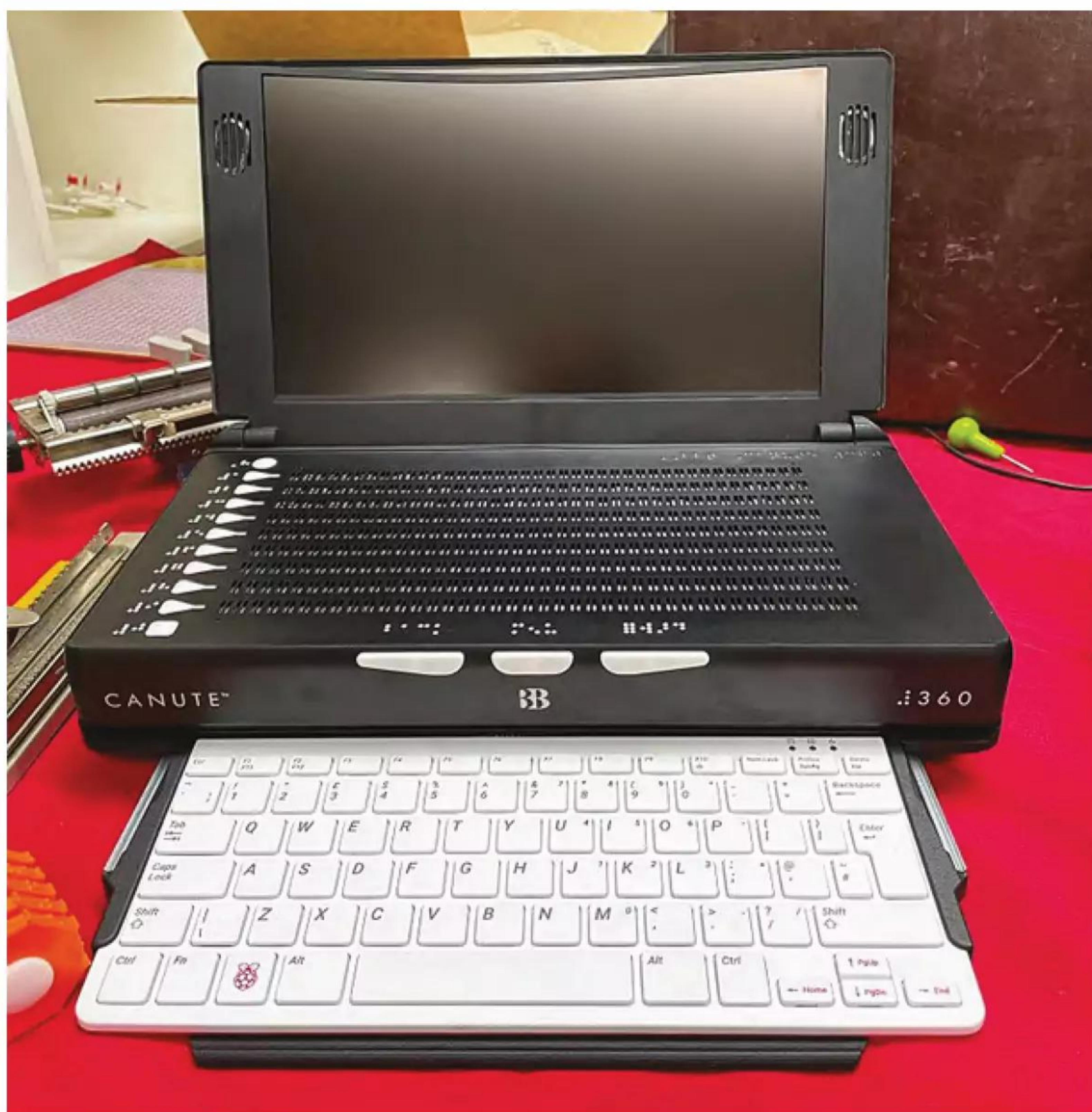
▲ The Canute Console Braille reader, based on Raspberry Pi, produces musical notation, charts, graphs, tables, and diagrams
