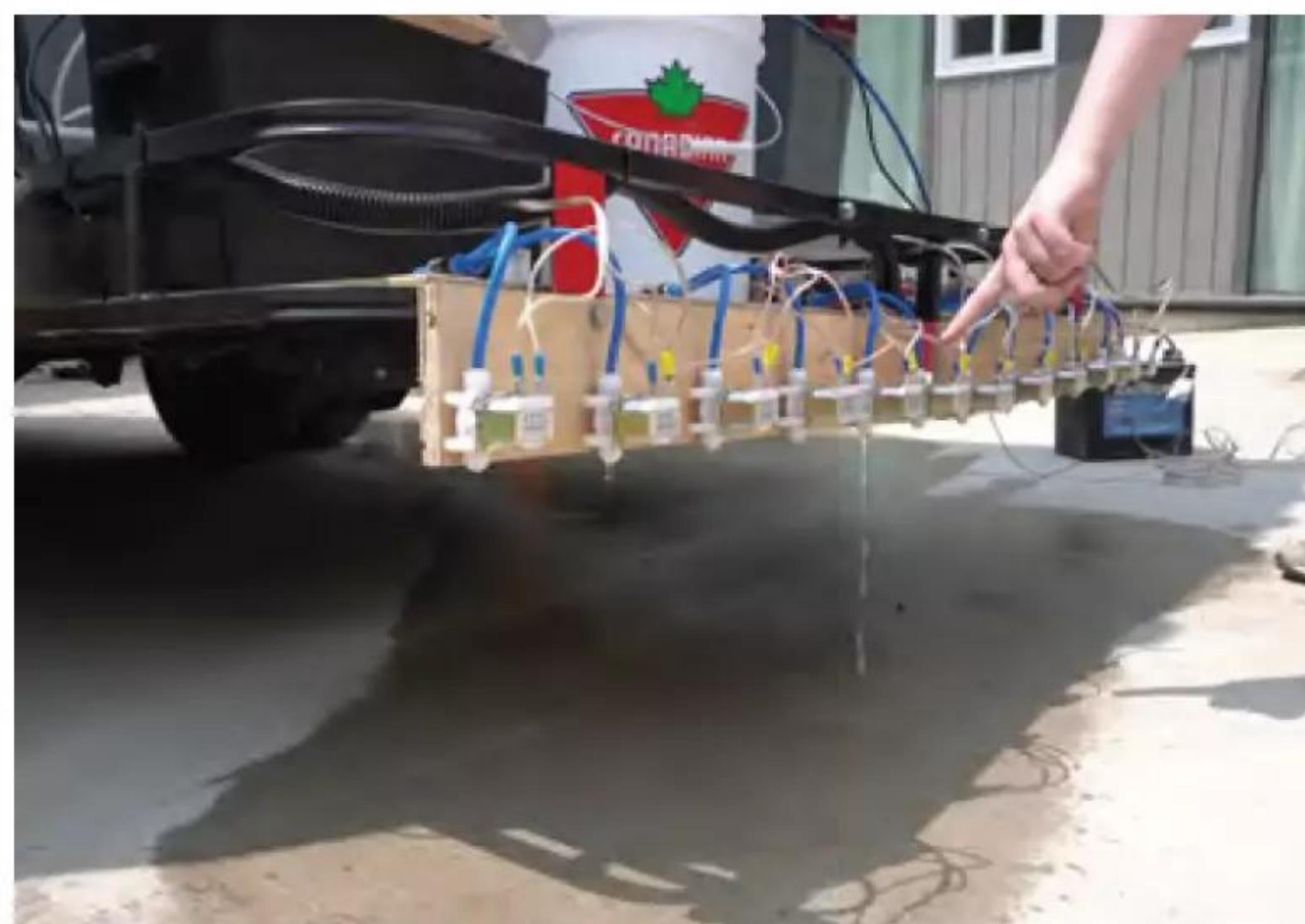
▲ Testing the solenoid valves in turn; each needs to dispense the correct amount of water
