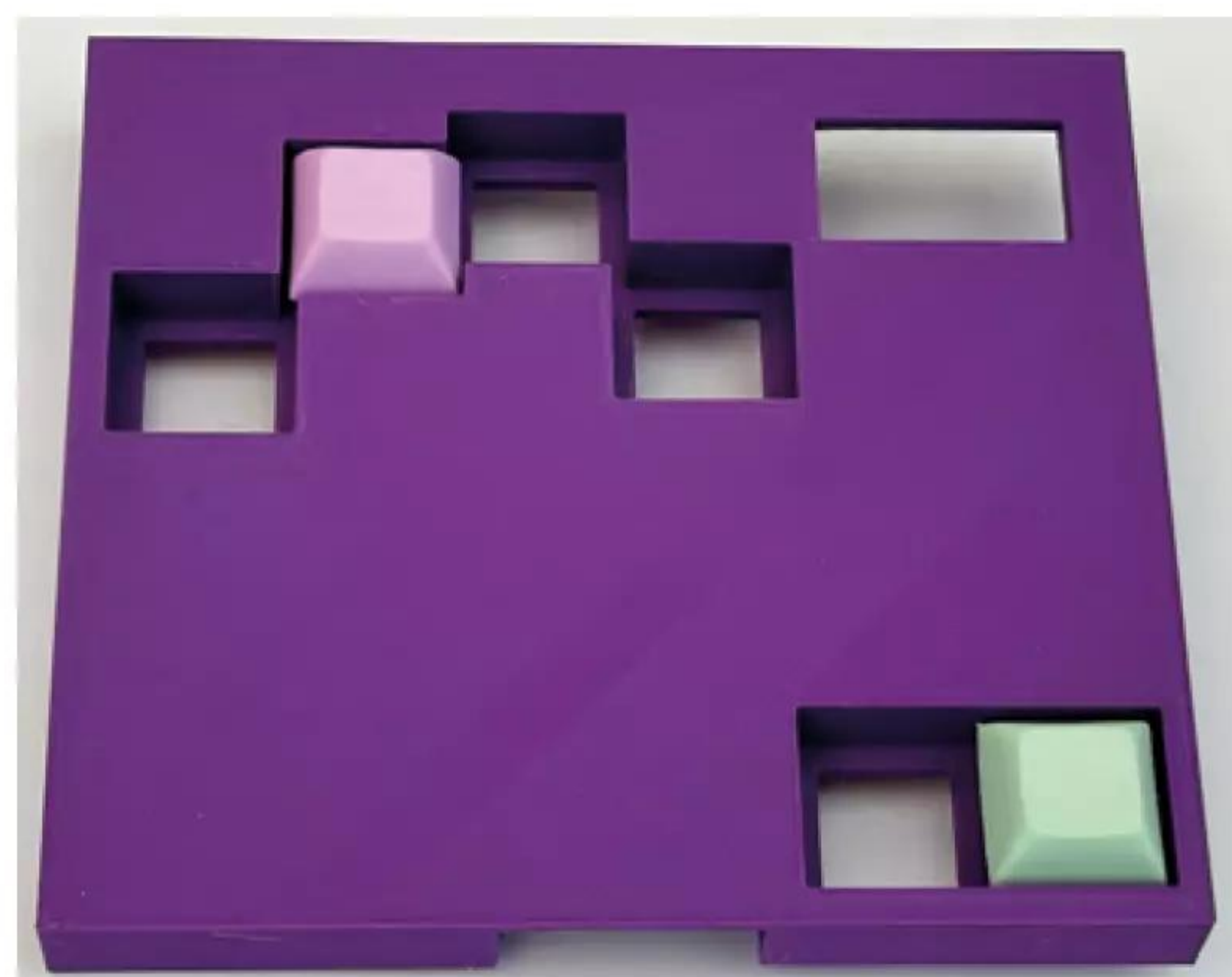
Figure 7 ♦ The keys snap into the holes in the front panel. They are not supported by the PCB underneath. They just plug into it
