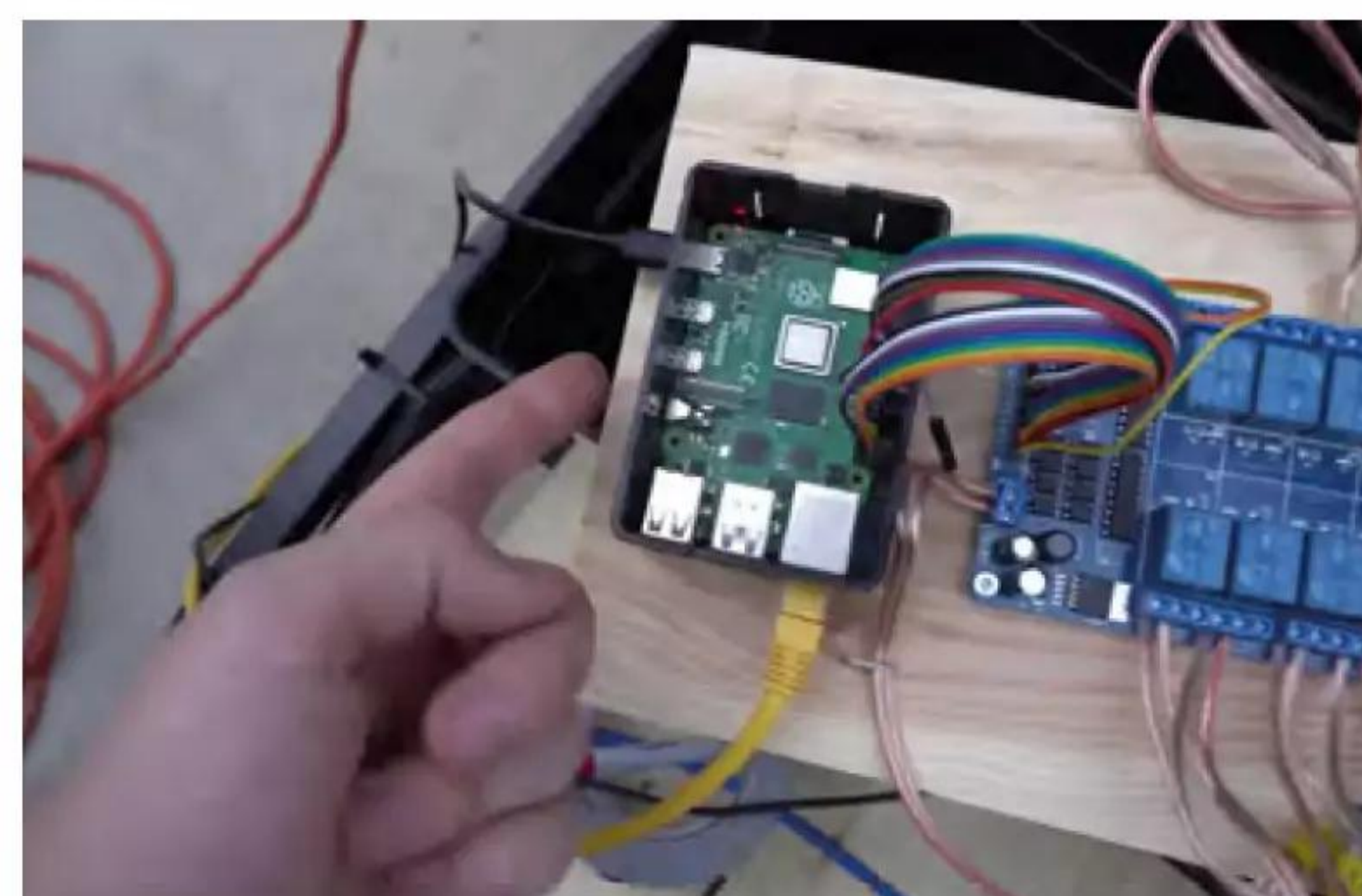
▲ A view of the inner workings, including a Raspberry Pi 4 and relay board
