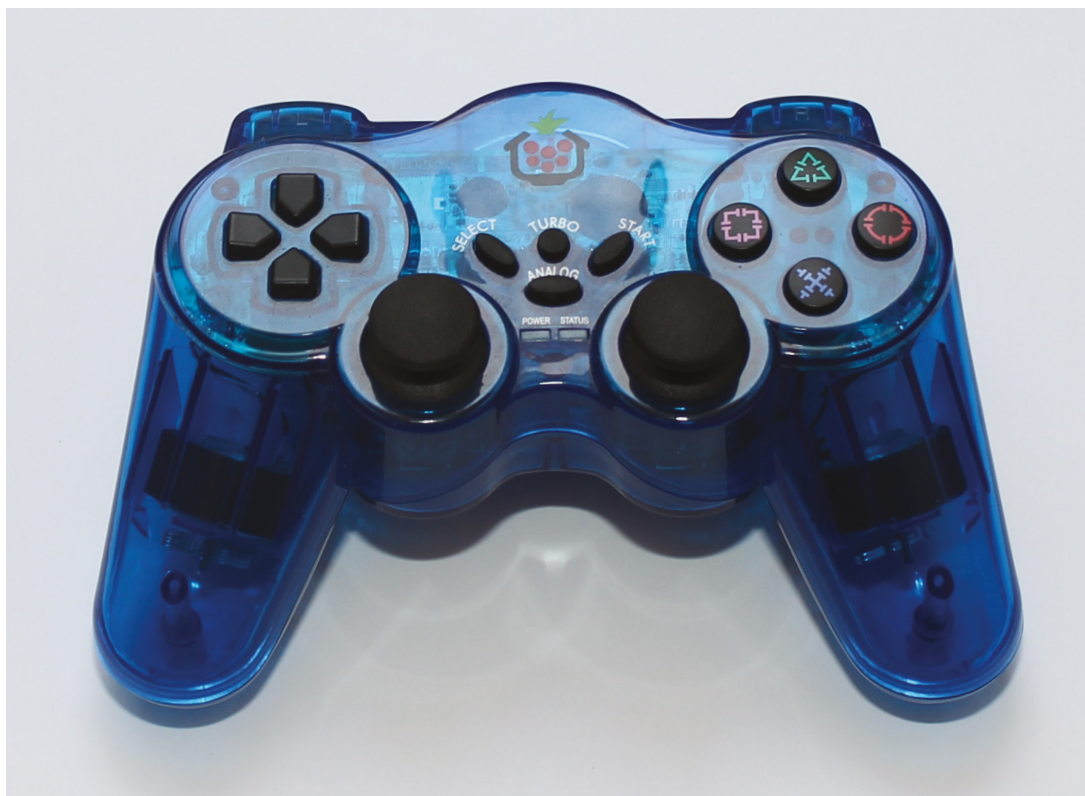
◀ Figure 5: A wireless USB gamepad. This is detected by Linux as an Xbox 360 controller
