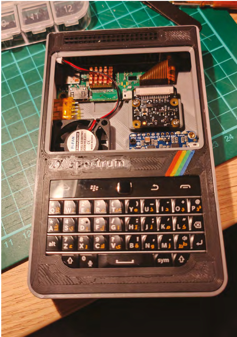
▲ The main components sit behind the screen. There is a 5V fan for cooling too
