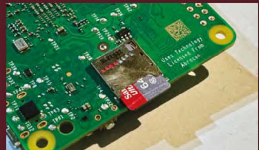
▲ SD cards are very fragile. Insert the card gently into the slot with the gold contacts facing the underside of the board
