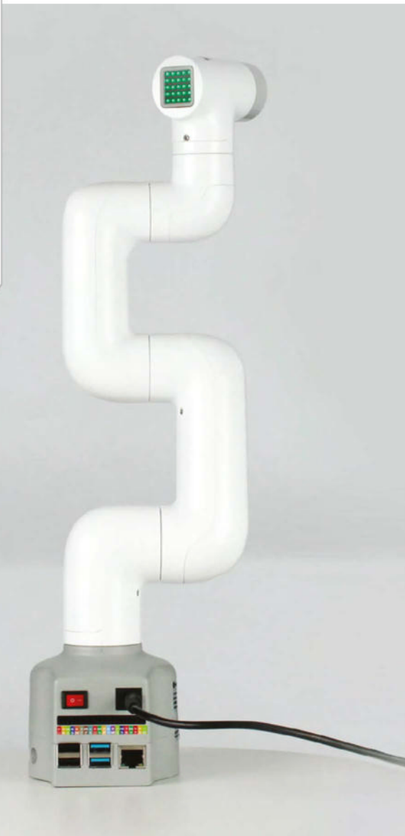
► The MyCobot 280 Pi robot arm extends to 350 mm at full height, but can also tuck up into a compact 'ball'
