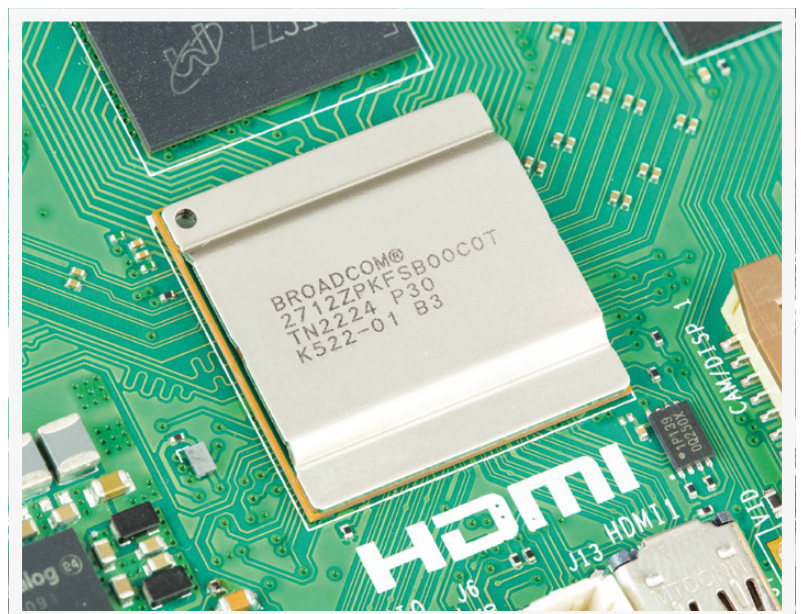
▼ Figure 2: Raspberry Pi’s system-on-chip (SoC)
