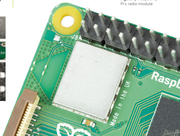
▼ Figure 4: Raspberry Pi's radio module
