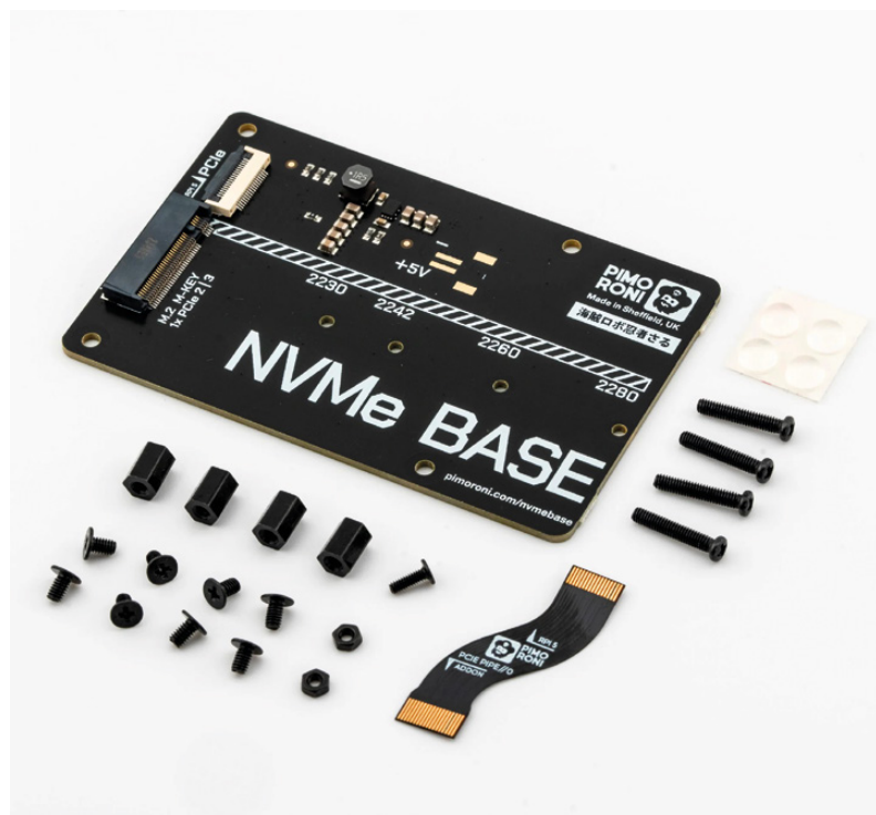
▲ The slimline NVMe Base fits snugly under Raspberry Pi 5, secured by bolts and standoffs
