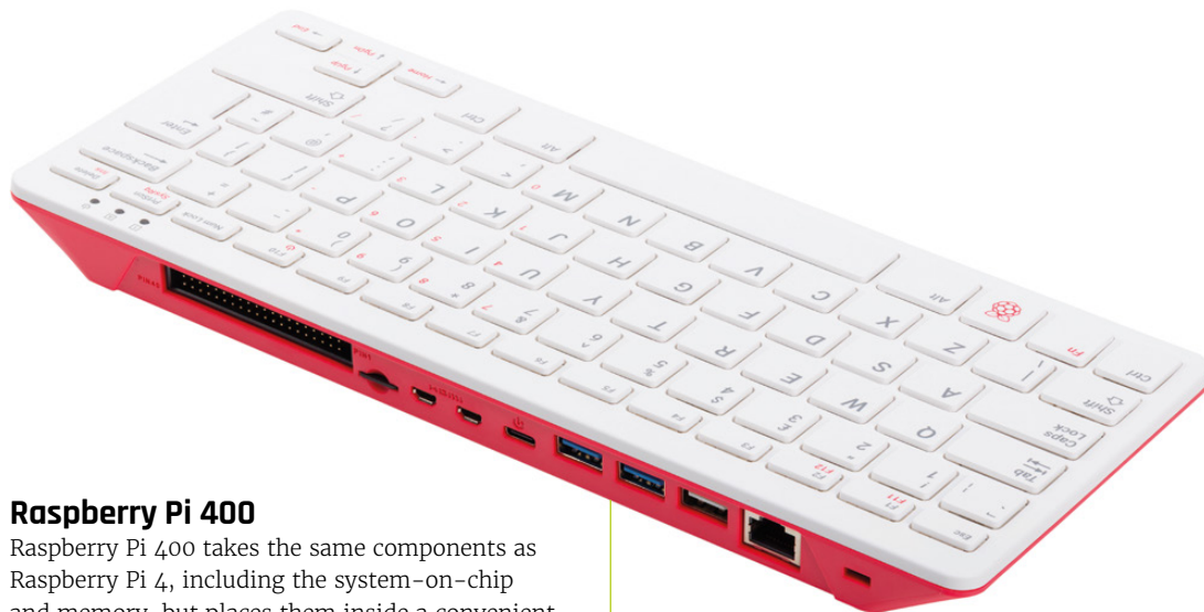
► Figure 18: The ports are found at the rear of Raspberry Pi 400
