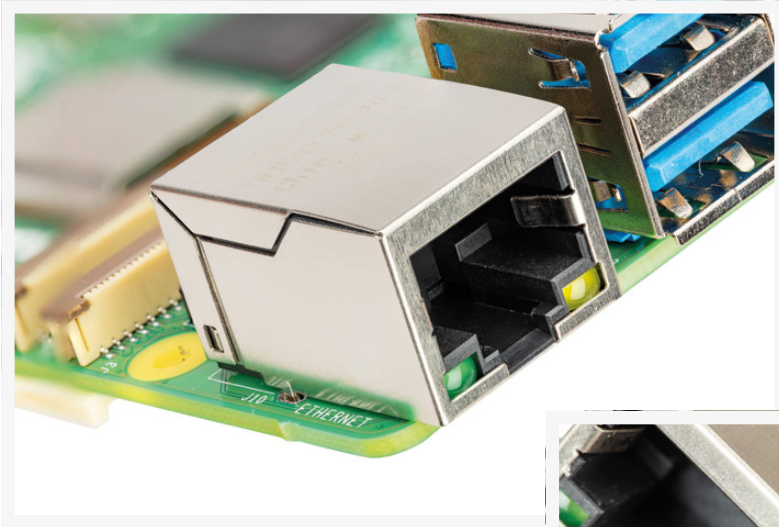
◀ Figure 8: Raspberry Pi's Ethernet port
