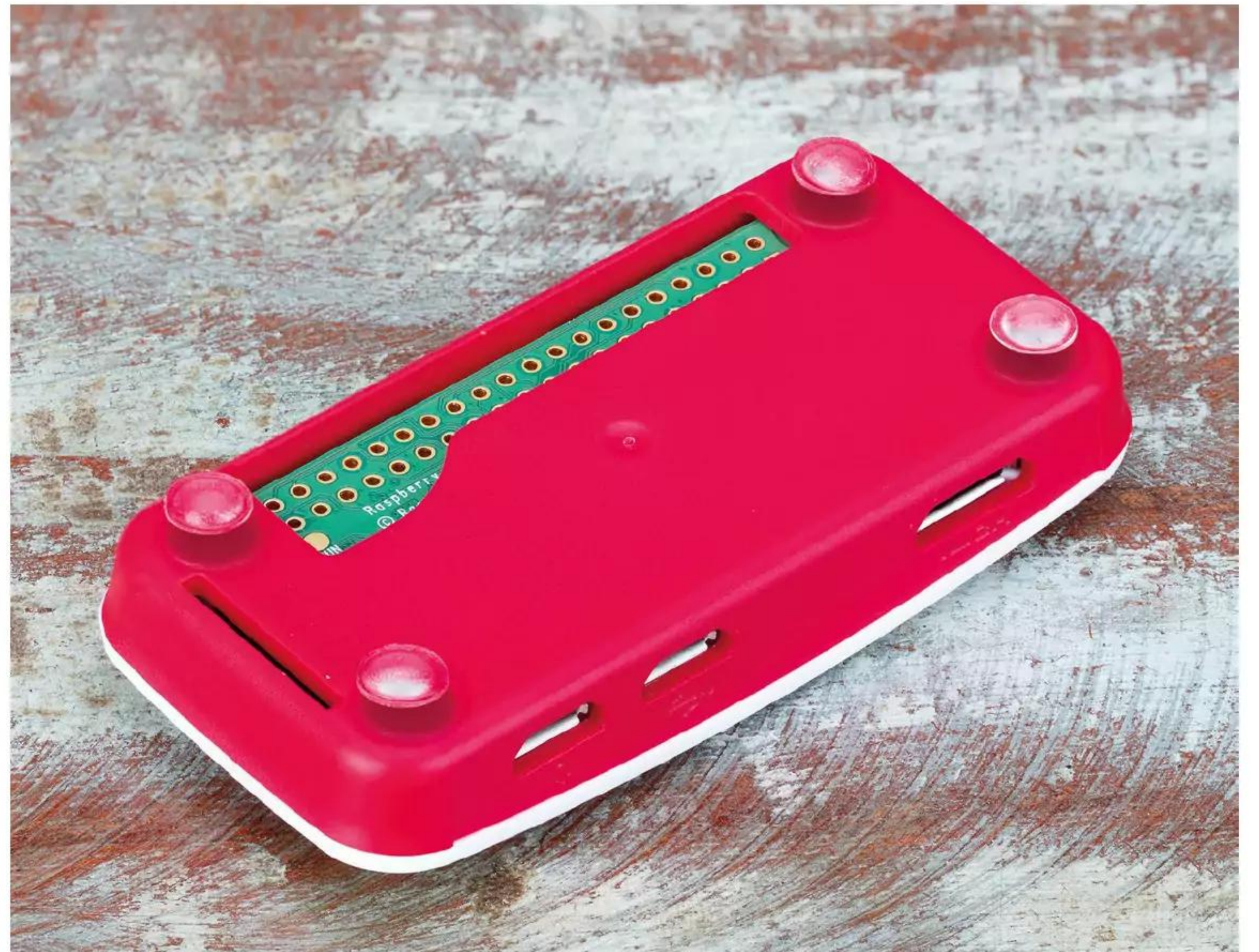
▲ Figure 12: Attaching the feet
