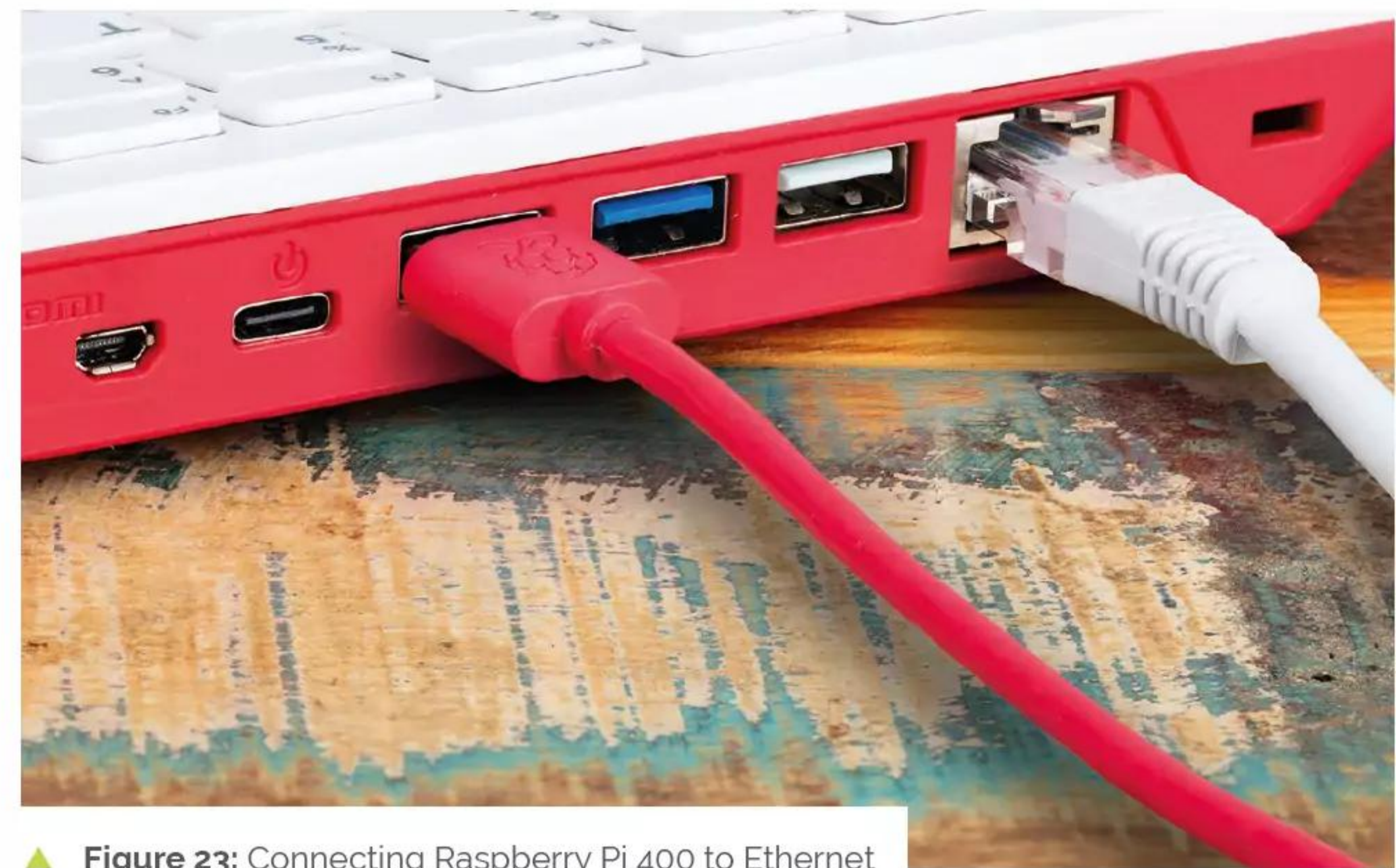
▲ Figure 23: Connecting Raspberry Pi 400 to Ethernet
