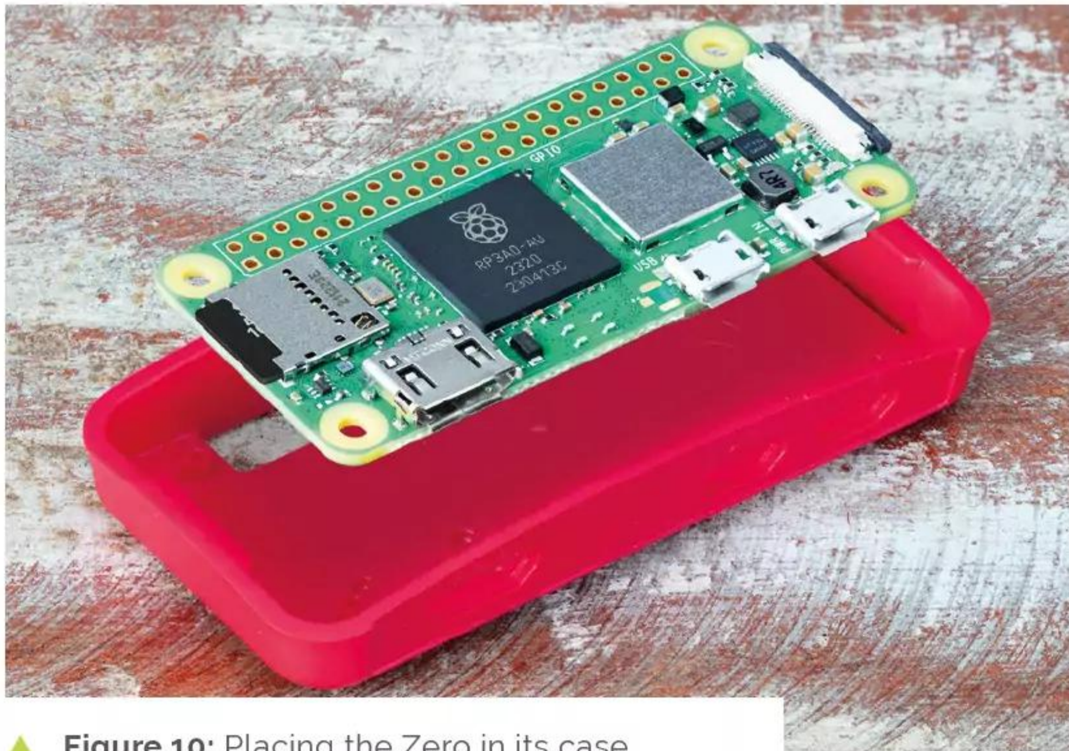
▲ Figure 10: Placing the Zero in its case
