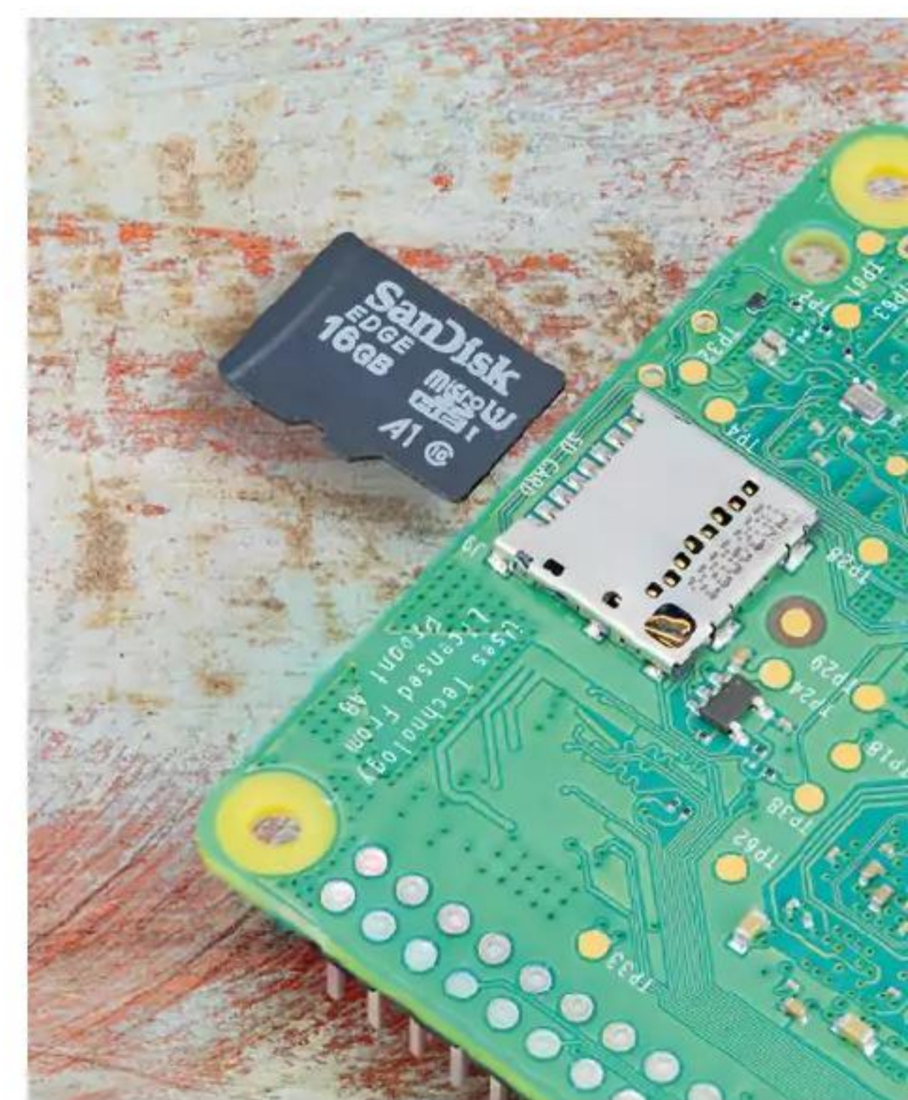
▼ Figure 13: Inserting the microSD card
