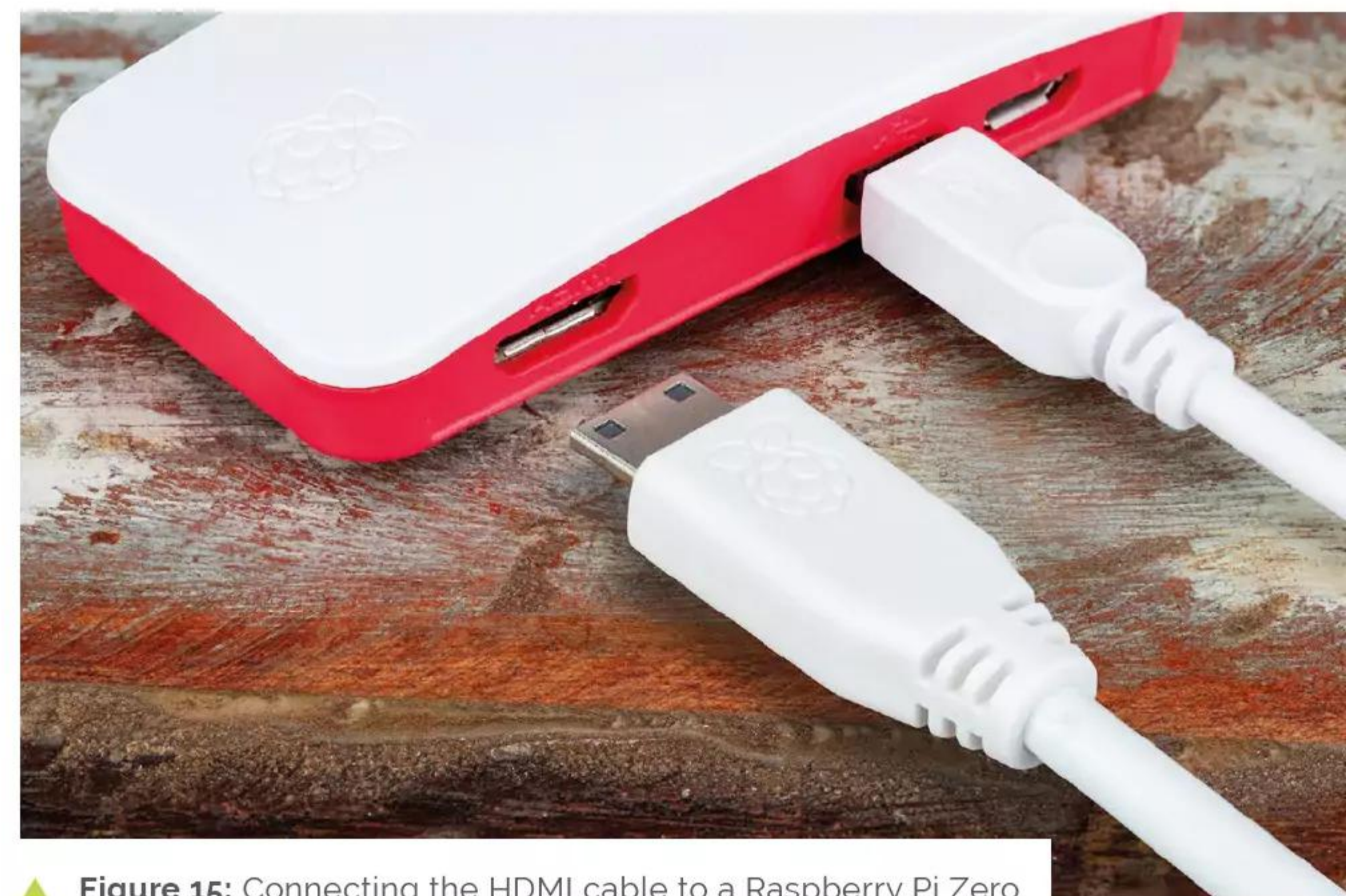
▲ Figure 15: Connecting the HDMI cable to a Raspberry Pi Zero
