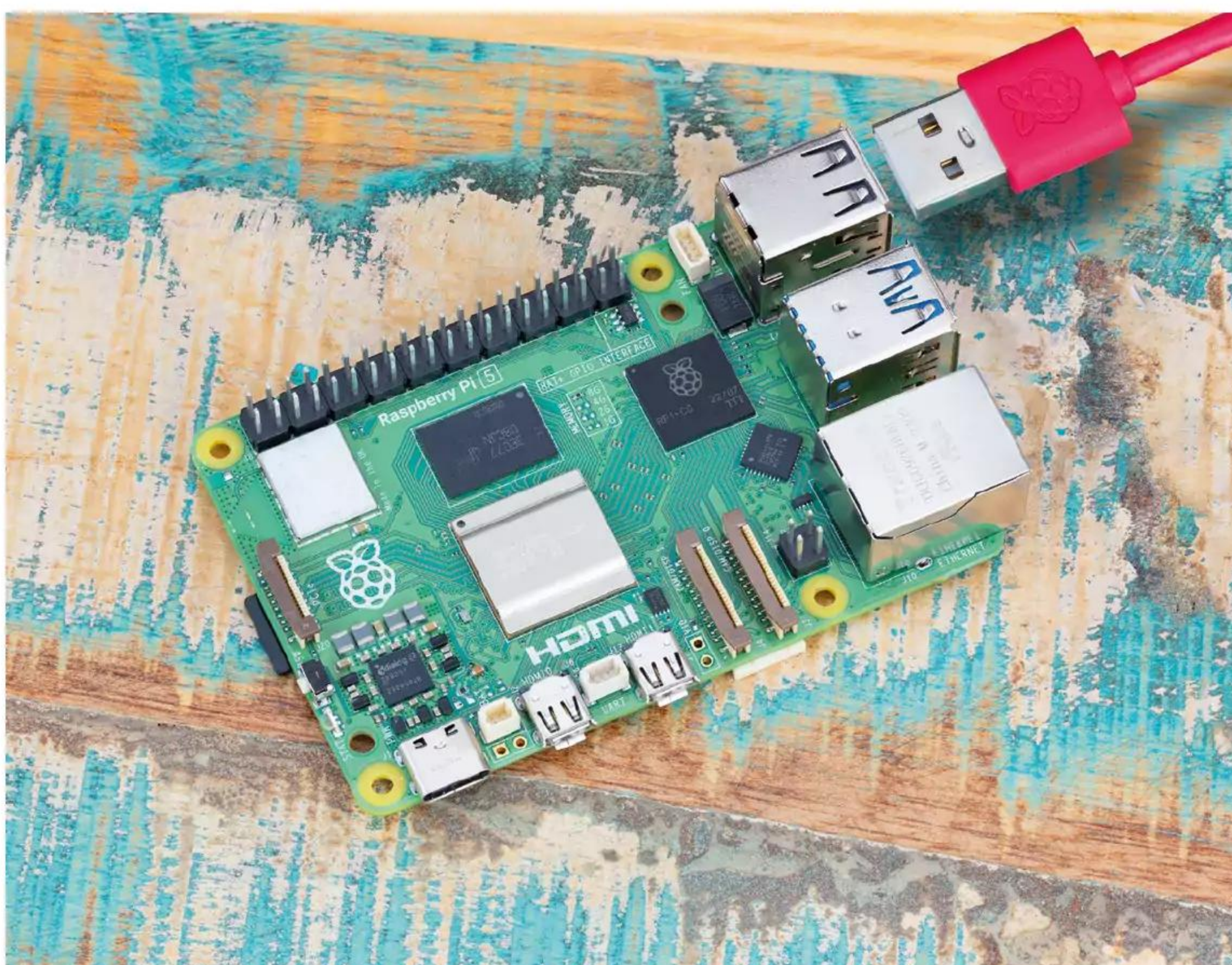
▼ Figure 14: Plugging a USB cable into a Raspberry Pi 5
