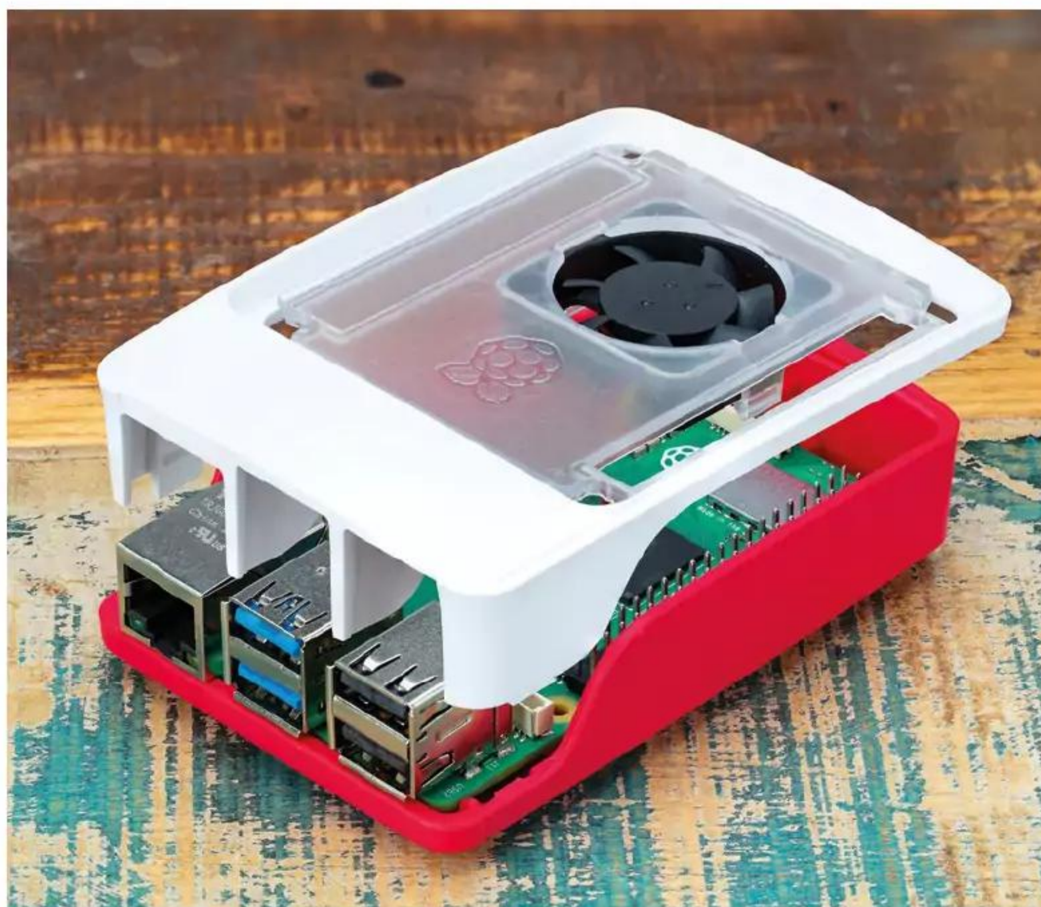
▲ Figure 8: Placing the lid on top of the case
