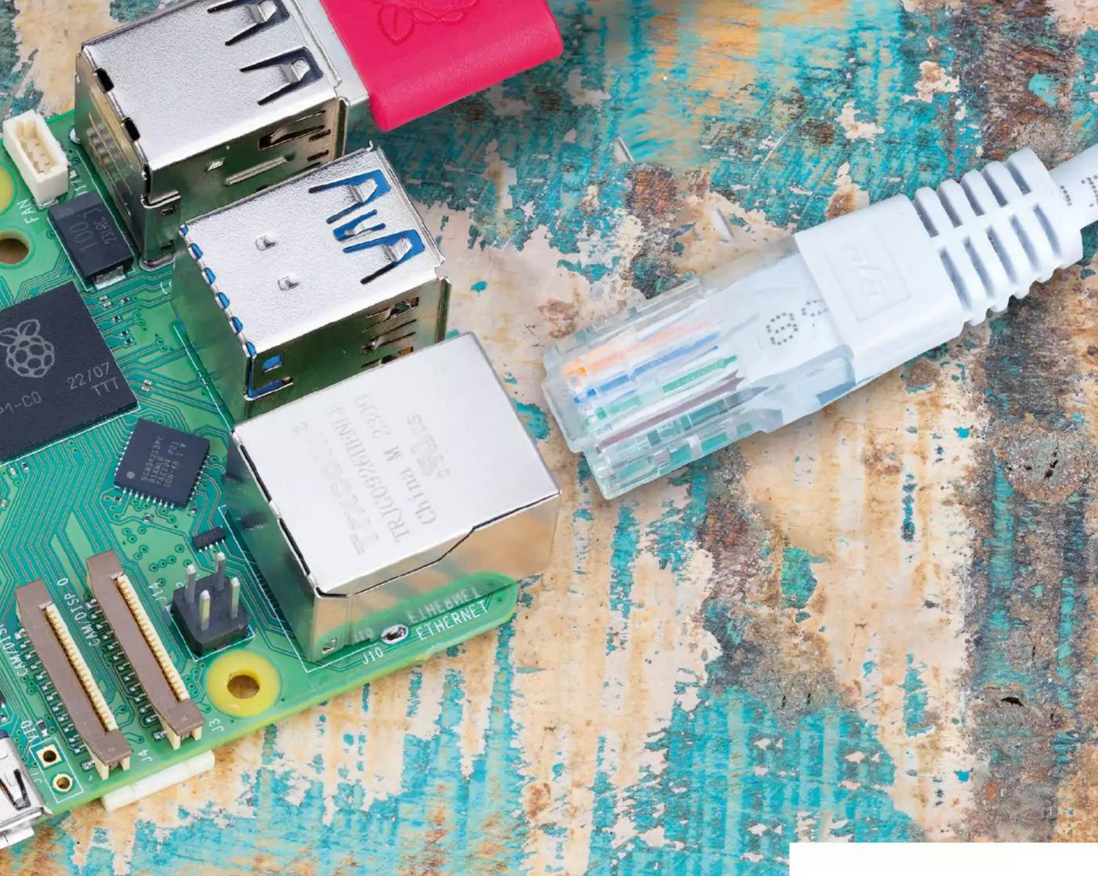
◀ Figure 17: Connecting Raspberry Pi 5 to Ethernet
