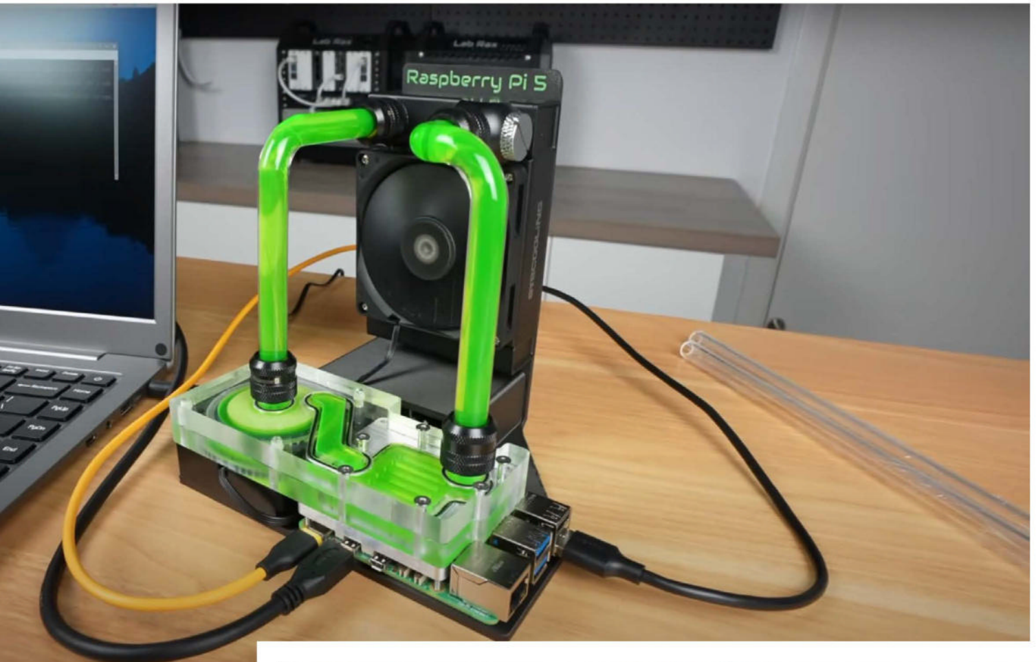
▲ Michael's homemade cooler keeps the Raspberry Pi 36 K (Kelvin) cooler than the equivalent setup using a Raspberry Pi Active Cooler
