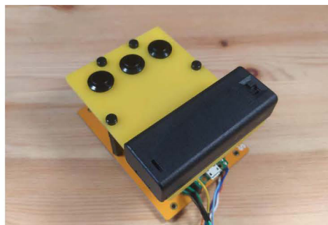
◀ Figure 6: Adding a small panel into which we mounted the buttons as a first attempt at a controller
