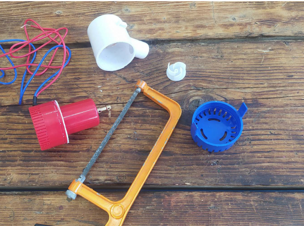
◀ Figure 5: Adapting a 1100 gallon per hour 12V bilge pump to become a thruster required cutting some case sections off the device
