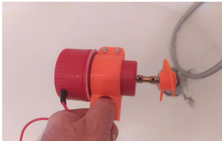
▼ Figure 6: A complete thruster with a DIY 3D-printed propeller mounted with an off-the-shelf brass coupler
