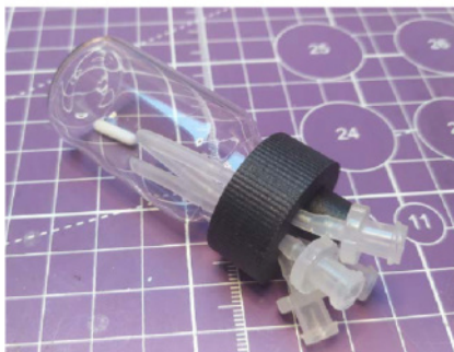
▲ Figure 1: The small 20ml glass vial allows for small samples and cultures to be grown
