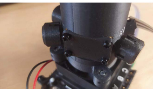
▲ Figure 4: A window in the chamber wall allows viewing, or is a place for add-ons like the Adafruit AS7341 spectrometry board
