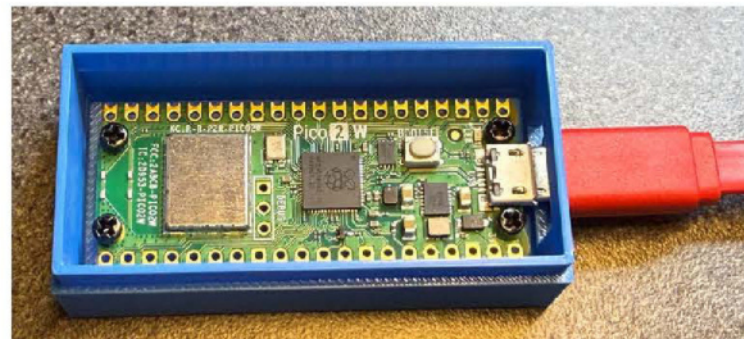
▲ The screws are M2 self-tapping, 4mm long
