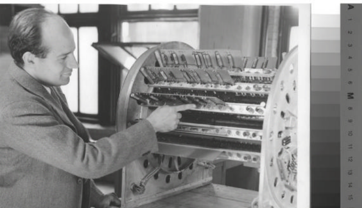
▲ Presper Eckert demonstrating a BINAC memory unit, c.1948-9 Image: courtesy of the Computer History Museum, CC BY-NC-SA
