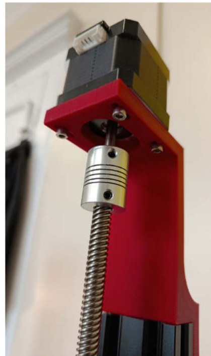
▼ Figure 2: The Nema 17 stepper motor mounts for the vertical axis were the first part we designed
