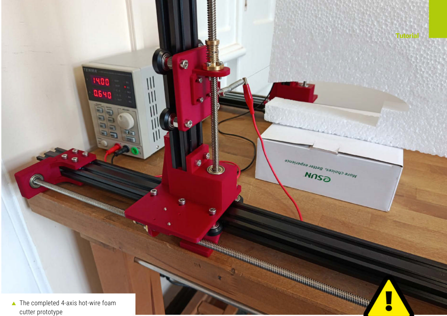
▼ Figure 2: The Nema 17 stepper motor mounts for the vertical axis were the first part we designed
