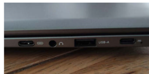
▲ Ports on the right-hand side include the USB-C power input, USB-A port, 3.5mm audio jack, and a full-featured USB-C port for connecting a smartphone
