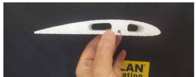
▲ Figure 6: Using a test G-code from RCKeith's site to cut a small section of a Clark Y aerofoil wing
