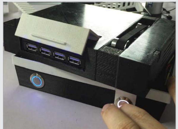
Above The flap is motorised, revealing the USB ports when turned on, thanks to a custom Python script
