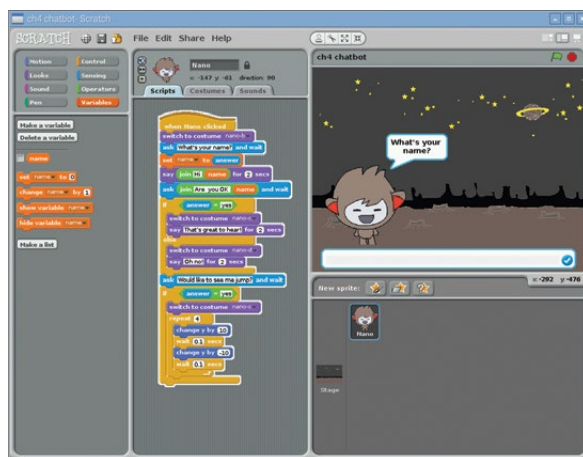
Above: We create a variable to store the user's name and then repeat it within Nano's speech
