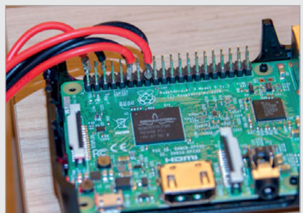
Above The power and data wires are soldered to the Raspberry Pi 3 and the software was installed to a 16GB card
