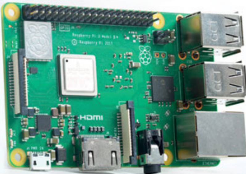
Above Nexmon SDR doesn't need any extra hardware for software-defined radio, just a Raspberry Pi B3+
