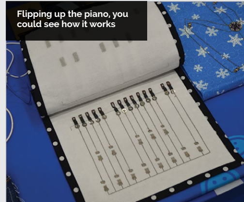
Below Brother was showing off projects using conductive thread, like this piano
