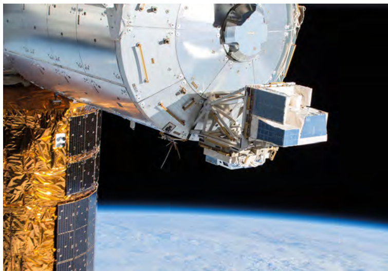
▲ The ARISS VHF antenna installed on the bottom of the Columbus module Credit: NASA/ESA
