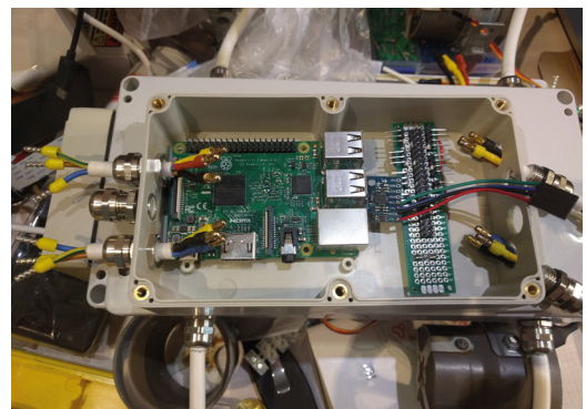
▶ The Raspberry Pi 3 sits in the housing and connects to a LiPo battery that also powers the LEDs and motors
