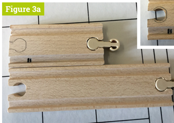
▲ Figure 3 Making the small track piece from a larger one
