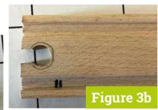
▲ Figure 3 Making the small track piece from a larger one
