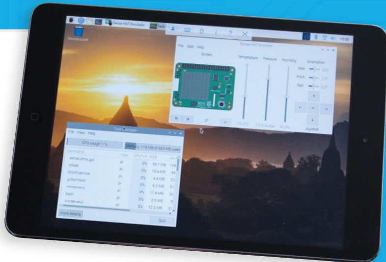
▲ Using VNC Viewer to manage Raspberry Pi from an iPad
