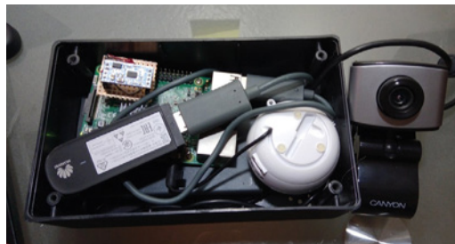
▲ A Raspberry Pi, powered by a battery pack, is connected to the camera, speaker, an accelerometer, and mobile data dongle
