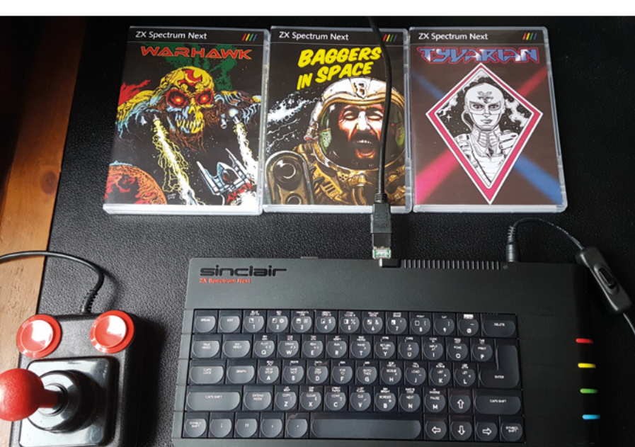
▲ Games made specially for the Next are saved as .NEX files which load directly to the computer via a SD card. Since the games are 768kB in size (or 1792kB for the 2MB models), it would take too long to route them via Raspberry Pi Zero
