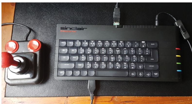
▲ The ZX Spectrum Next contains a Z80 processor on an FPGA, 1MB of RAM expandable to 2MB, hardware sprites, 256 colours, RGB/VGA/HDMI video output, and three AY-3-8912 audio chips
