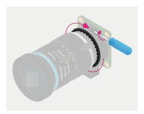
**Back focus adjustment ring** 03 The back focus adjustment ring should be screwed in fully. Tighten the back focus lock screw to make sure it does not move out of this position when adjusting the aperture or focus.
