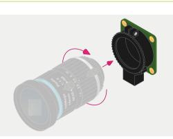
Fit the lens to the camera 02 Rotate the lens and C-CS adapter clockwise all the way into the back focus adjustment ring.
