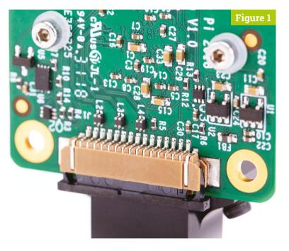
If using a Raspberry Pi Zero, its Camera port is found on the edge of the board. However, as it's a smaller size than the regular one on other Raspberry Pi models, you'll need a camera adapter cable to use it (magpi.cc/zerocamcable).
