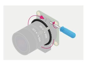
**D2 Back focus adjustment ring** The back focus adjustment ring should be screwed in fully for the shortest possible backfocal length. Tighten the back focus lock screw to make sure it does not move out of this position when adjusting the aperture or focus.
