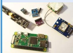
Connect your Raspberry Pi Zero to an nRF24L01+ transceiver. This will receive the data from the other sensors. You also need a u-blox NEO-6 GPS receiver to obtain GPS readings.
