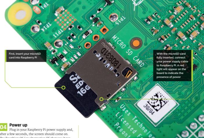
after a few seconds, the screen should come on. The Raspbian OS (or alternative OS that you have installed to the microSD card) will then boot up.
