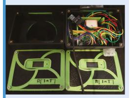
**D2** Temperature, pressure, humidity, and light readings are provided by BME280 and BH1750 sensors. Data from all the sensors and transceivers is stored locally in an SQLite database on Raspberry Pi Zero.
