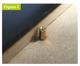
Figure 2 Using a bent solder tag to push out the sides and stop them bending
