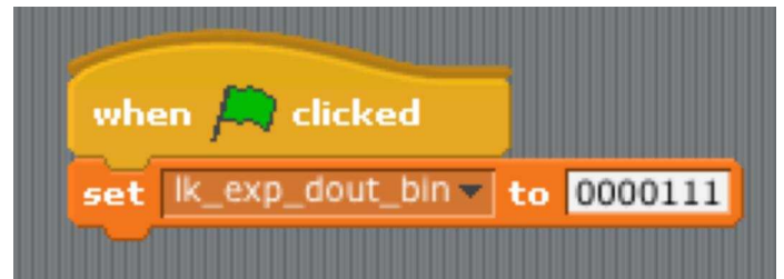
Figure 5.0 – Writing to the digital outputs in Scratch
