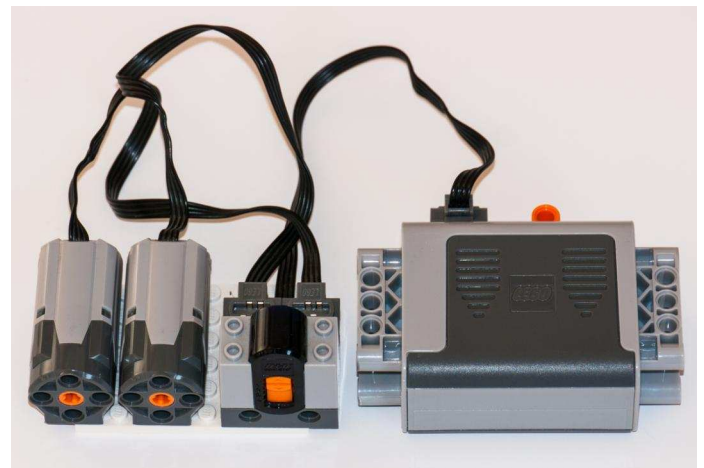
Figure 1 - Some LEGO® Power Functions Components left to right: Motors, IR Receiver, Battery Box
