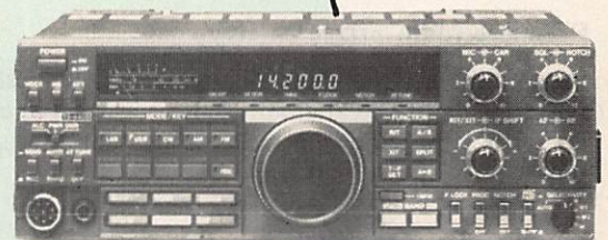
TS 440 SP SSB-AM-FM-RTTY 100 KHz-30 MHz-100 W HF
