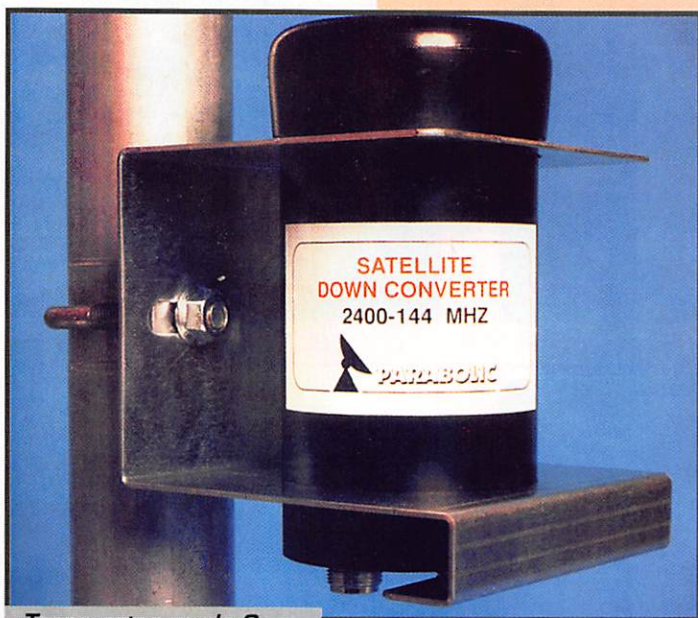
Transverter mode S 2400 → 144 MHz.
