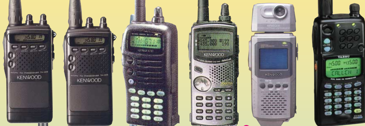
KENWOOD TH 22 VHF KENWOOD TH-42 UHF TH-G71 Bibande KENWOOD TH-D7 2 Bibande KENWOOD VC-H1 YAESU FT-51 Bibande
